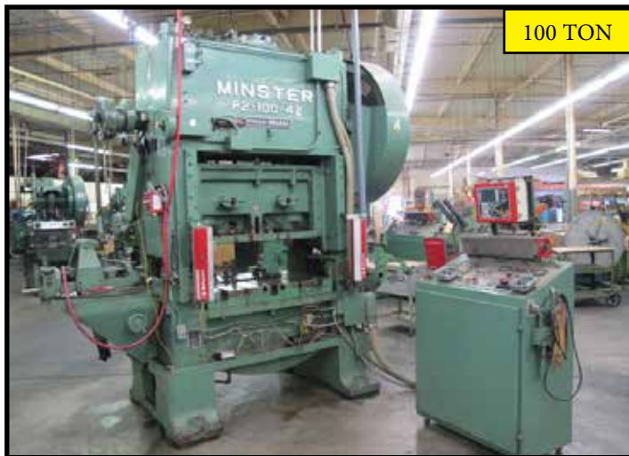
Minster P2-100-42 "Piece Maker" 100-Ton Straight Side Stamping Press w/ Minster Controls, Honeywell SmartPAK Wintriss Press Automation System, Wintriss Load Analyzer, Wintriss DS12 Sensor Input Module, Shadow IV Light Curtain, Air Clutch
