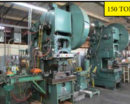
Verson 7 1/2 OBG 105-Ton Open Back Gap Stamping Presses w/ Air Clutch, 8" Stroke, 4" Slide Adj, 18" Shut Height, 35 Strokes/Min, 30" x 39" Bolster, Verson Type K1614-4 17.7-Ton Cushion
