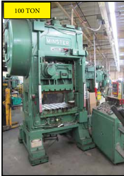
Minster P2-100-42 "Piece Maker" 100-Ton Straight Side Stamping Press w/ Minster Controls, Data Instruments DiPRO 1500 Wintriss Die Protection, Wintriss Load Analyzer, Shadow VII Light Curtain, Air Clutch, Counterbalance 97 Sq/In, 0-300 Strokes/Min
