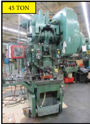
Bliss C45 45-Ton OBI Stamping Press w/ Data Instruments SmartPAK Wintriss Press Automation System, Air Die Balance, Air Clutch
