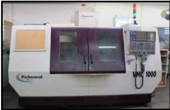
Richmond VMC 1000 CNC Vertical Machining Center w/ Fanuc/Richmond Controls, 20-Station ATC, CAT-40 Spindle, 8000 RPM
