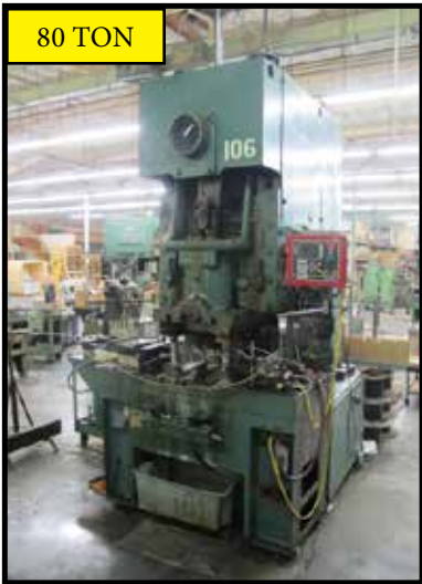
Aida 8 mdl. C1-8(1) 80-Ton Stamping Press w/ Data Instruments SmartPAK Wintriss Press Automation Controls, DiPRO Sensor Interface, Programmable Cam Outputs, Die Weight Air Balance, 40-115 Strokes/Min
