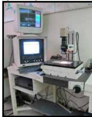
ROI OMIS II Video Inspection System w/ ROI Optical Video
