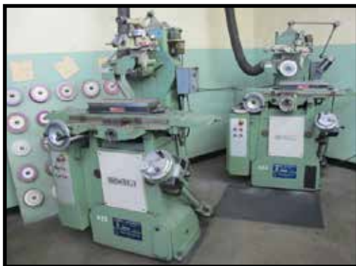
Jones-Shipman 540H 6" x 18" Automatic Surface Grinders w/PG Ltd Optical Dressers
