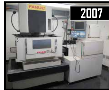
2007 Fanuc Robocut α-1iC CNC Wire EDM Machine w/ Fanuc Series 180is-WB Controls, Hand
