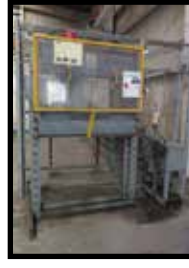
Nugier H80-14 80 Ton Sliding Ram Electric/ Hydraulic H-Frame
