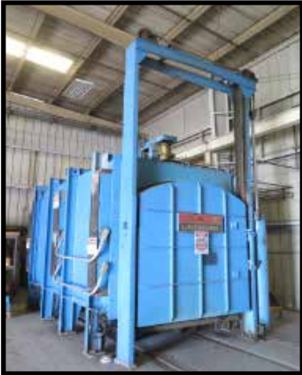
Lindberg type 13-20-601248-18CBS Homogenizing Oven w/ 179kW, 1850 Degree Max Temp
