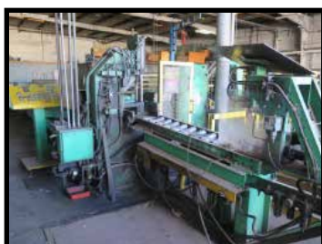
Oliver 36" Automatic Billet Saw w/ Allen Bradley PanelView 1000 PLC Controls
