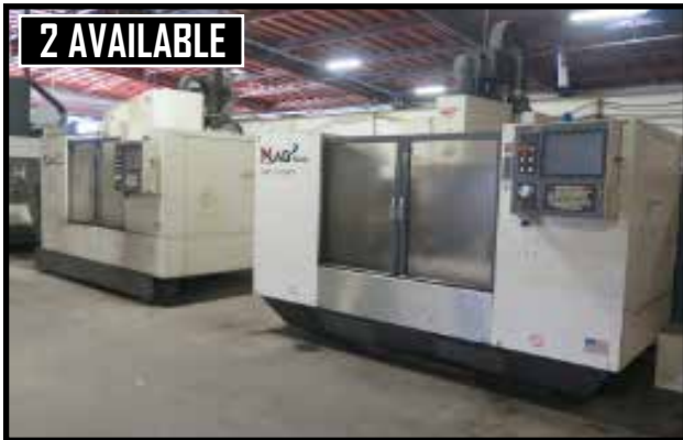
MAG Fadal VMC4020 FXMP HT CNC Vertical Machining Centers w/ MultiProcessor CNC Controls, CAT-40, 10,000 RPM
