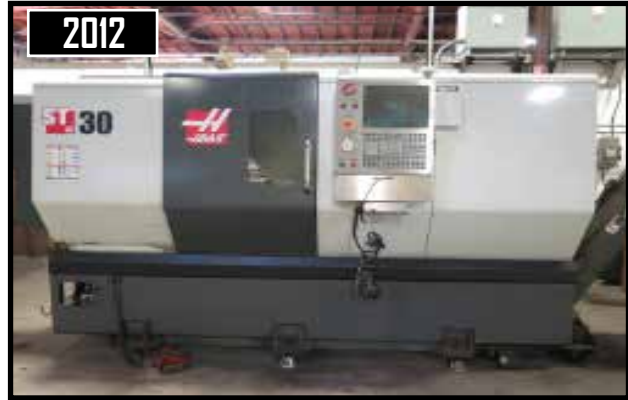
12/2012 Haas ST-30 CNC Turning Center w/ 12-Station Turret, 3200 RPM, Rigid Tapping
