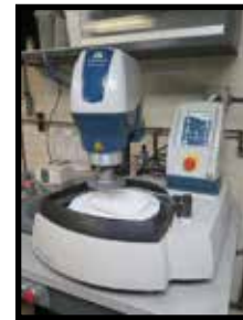
2010 Buehler AutoMet 250 mdl. 49-7210 Automatic Sample Preparation Grinder - Polisher
