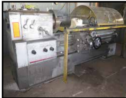
Lion C11MS80 20" x 72" Gap Bed Lathe w/ Tailstock, 12" 3-Jaw Chuck
