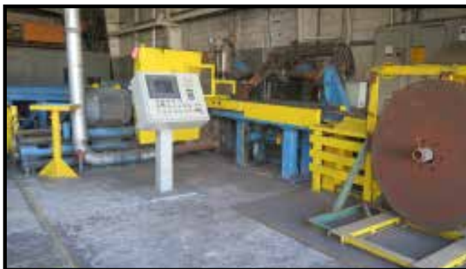
Oliver 52" Automatic Billet Saw w/ Allen Bradley PanelView 1000 PLC Controls
