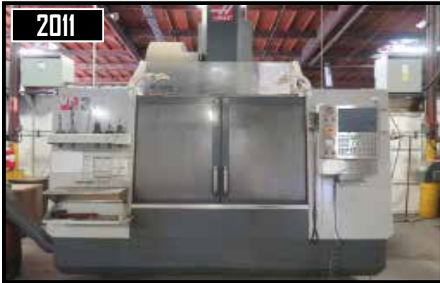
10/2011 Haas VF-3YT/50 CNC Vertical Machining Center w/ 30-Station Side Mounted ATC, CAT-50
