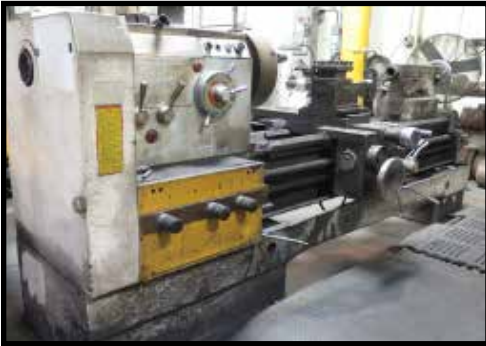
Lion C10TM 29" x 67" Gear-Gap Bed Lathe w/ 30-1500 RPM, 4" Thru Spindle Bore, Taper Attachment
