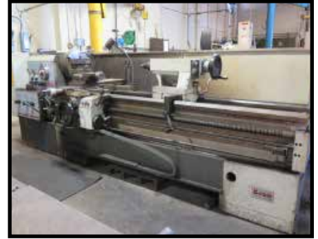
Lion C10MS 26" x 90" Gear-Gap Bed Lathe w/ 10-1500 RPM, 4" Thru Bore, Inch Threading, Tailstock
