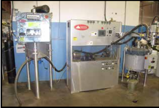
TRICO POLY SYSTEM POLYURETHANE PROCESSING LINE W/ SL DG CONTINOUS SLINGER DEGASSER, MKXX HYDRODESPENSER, BATCH MIXER.
