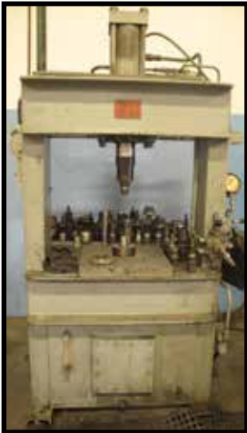
KARD 30 TON HYDRAULIC H FRAME PRESS.
