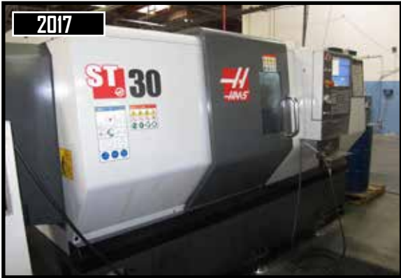
2017 HAAS ST30 CNC LATHE, 10" CHUCK, 3400 SPINDLE SPEED, , 33.75" SWING, S/N3107018.
