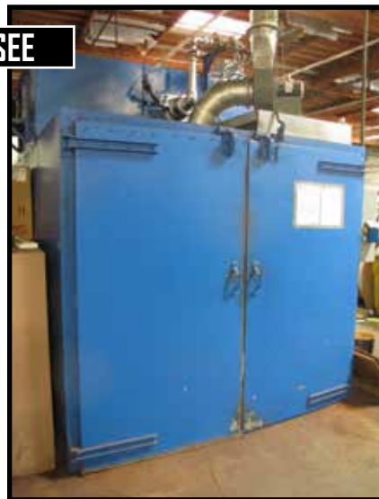
E.J. CALLAHAN MODEL 6612 500 F WALK IN OVEN W/ DOUBLE DOORS, 5' X 10' WORK AREA, 450,000 BTU.
