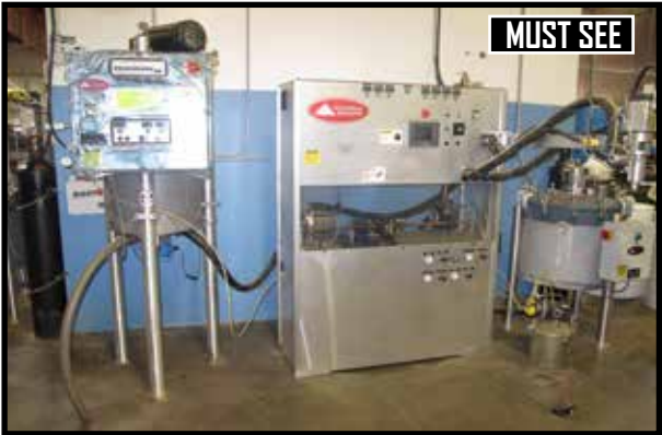
TRICO POLY SYSTEM POLYURETHANE PROCESSING LINE W/ SL DG CONTINUOUS SLINGER DEGASSER, MKXV HYDRODESPENSER, BATCH MIXER.
