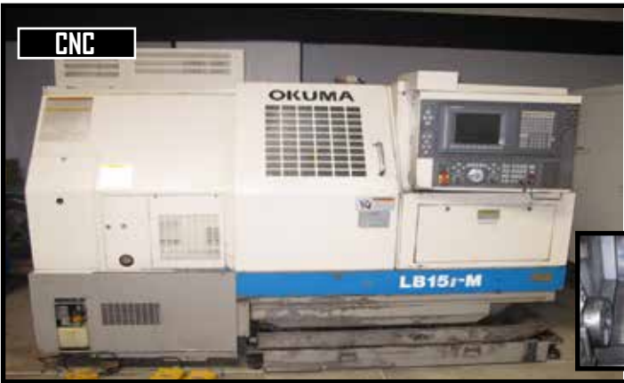
OKUMA LB15II-M CNC LATHE W/ LIVE TOOL MILLING, 10" CHUCK, OSP-U100L CONTROL, S/N 3090.
