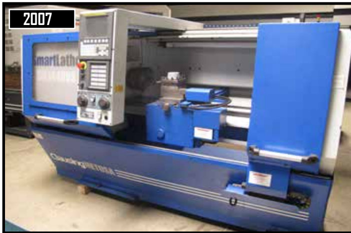
2007 CLAUSING-METOSA SM1440VS SMART 180 CNC FLAT BED LATHE W/ FANUC Oi MATE-TC CONTROL, 8" CHUCK, S/N 53551.
