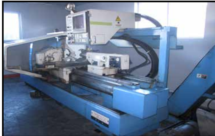
MAZAK M5-N FLAT BED LATHE, W/ T32-2 CONTROL, 12" CHUCK, 8 POS TURRET, CHIP CONVEYOR.
