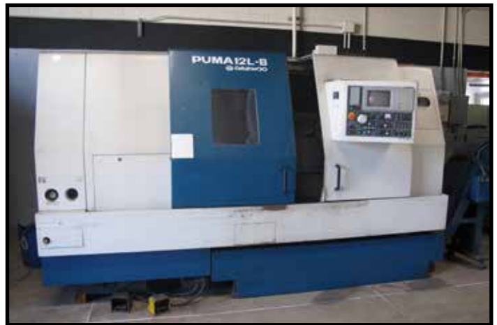
DAEWOO PUMA 12L-B CNC LATHE, 15" CHUCK, 12 POSITION TURRET, MITS CONTROL, S/N PL121101.
