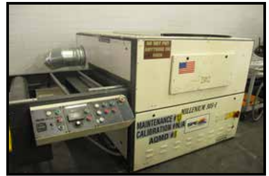
MILLENIUM-305-1 30" UV CURING OVEN.
