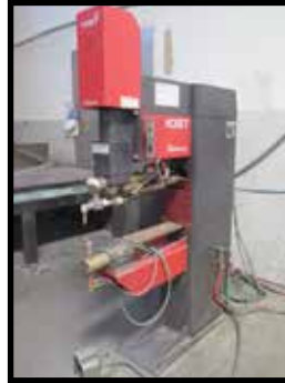
2000 Amada ID-40-ST 80kW Spot Welder w/ Amada DIT-453 EA-1 Controls
