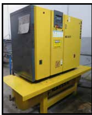
2006 Kaeser AS20T 20Hp Rotary Air Compressor
