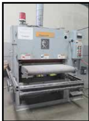
Timesavers mdl. 137-1HDMES 37" Belt Grainer
