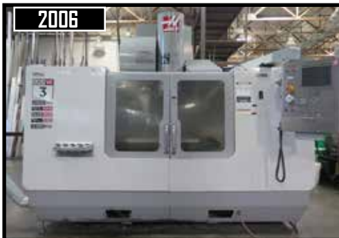
2006 Haas VF-3SSYT 4-Axis CNC Vertical Machining Center w/ Haas Controls, 24-Station Side Mounted ATC, CAT-40 Spindle, 12,000 RPM
