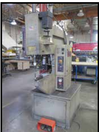
Haeger 8 Ton x 24" Hardware Insertion Press
