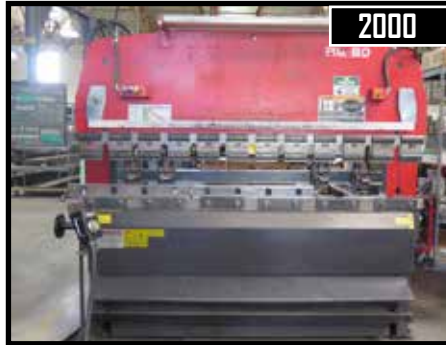
2000 Amada RG-80 80 Ton x 8' CNC Press Brake w/ NC9-EX II Controls
