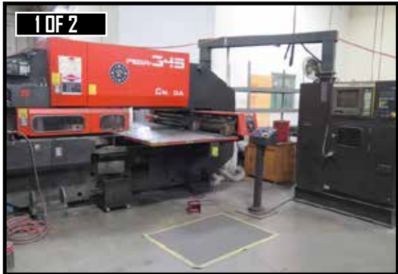
Amada PEGA 345 30 Ton 58-Station CNC Turret Punch Press w/ O4P-C Controls
