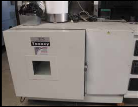
TPS Tenney mdl. BTRC -70 Deg C to 200 Deg C Thermal Chamber 0801000056 w/ TenneyVersaTenn II Digital Controls, Chart Recorder.
