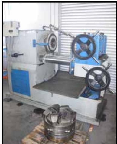
6" Power Pipe Threader w/ 16" Threading Heed 7" Thru Head.
