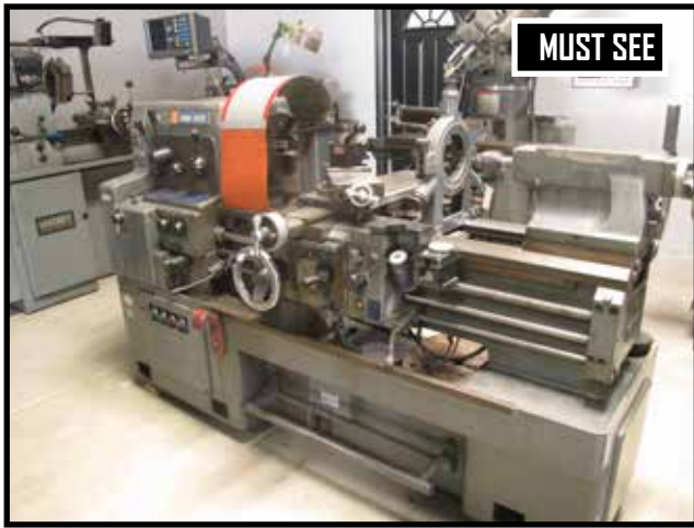
Mori Seiki MS-850G 16" x 36" Geared Head Gap Bed Lathe s/n 11721 w/ Acu-Rite Programmable DRO, 32-1800 RPM, Inch Threading, Tailstock, Trava-Dial, Aloris Tool Post, Coolant.
