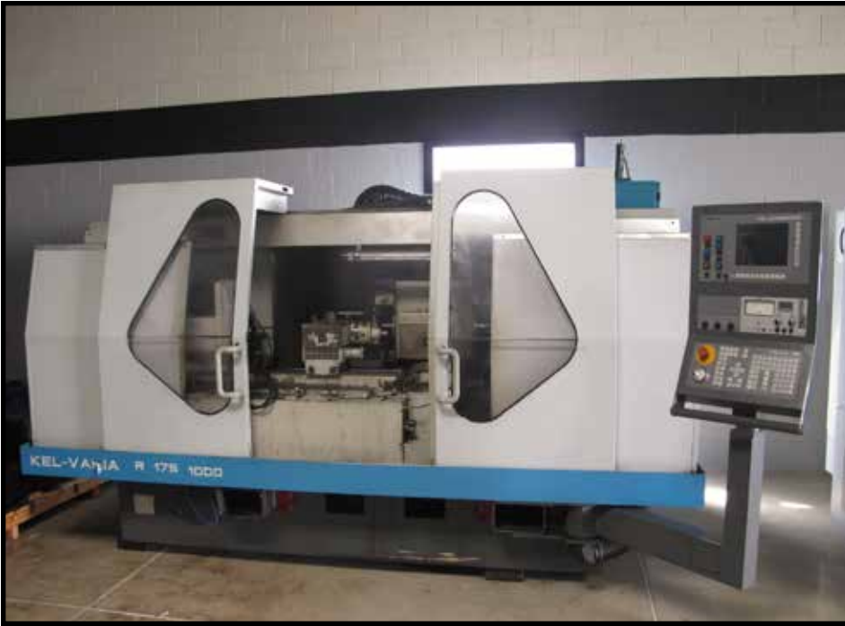
Kellenberger "Kel-Varia R175/1000" CNC Cylindrical Grinder s/n 650296 w/ Kelco 90 CNC Controls, 1000mm (39.4") Between Centers, Auto Sizer Head, 10 Deg Tilt Table, Coolant.
