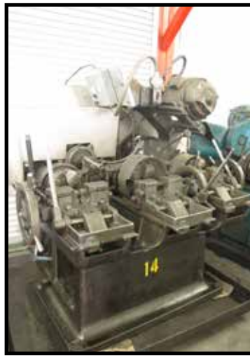
Landis 3-Head Power Pipe Threader w/ 9" threading Heads, 2" Thru Head.
