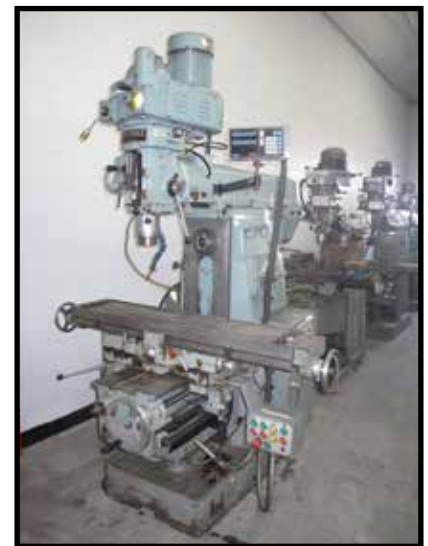
Supermax Series II mdl. YC2GUS Universal Mill s/n 04804 w/ Sony Millman DRO, Mitutoyo Digital "Z" Scale, 75-4220 Vertical RPM, 40-Taper Spindle, 49-1300 Horizontal RPM, 40-Taper Spindle, BoxWays, Power Feeds, 11" x 51" Table.
