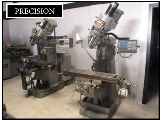
2) Bridgeport Vertical Mills, 2hp, Dro and P.F. Table.
