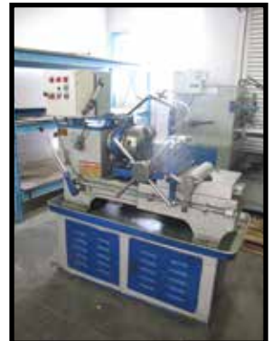
IMC Industrial Machinery Corp. mdl. 2015 Power Pipe Threader s/n 4323 w/ 60-90 RPM, 2-Speeds, 9" Threading Head, 1.5" Cap.
