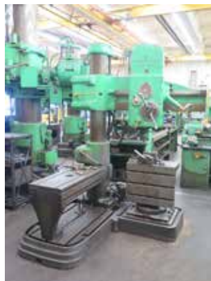
American Hole Wizard 9" Column x 3' Radial Arm Drill
