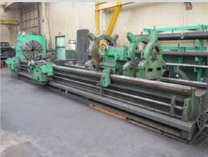
Monarch Series 91 mdl. 4025 40" x 252" Engine Lathe
