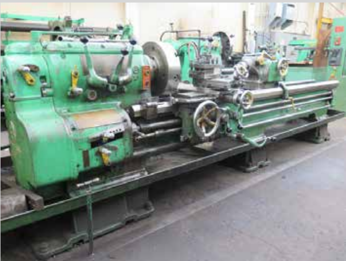
Axelson 18 18" x 103" Geared Head Lathe
