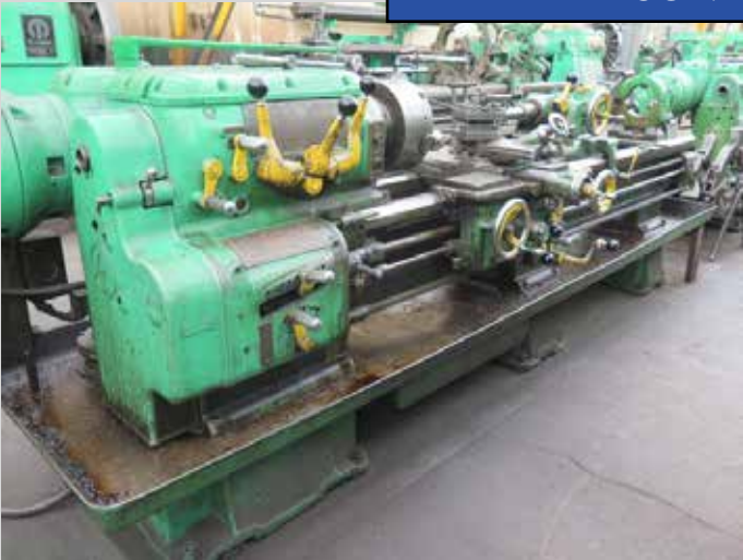
Axelson 16 16" x 80" Geared Head Lathe
