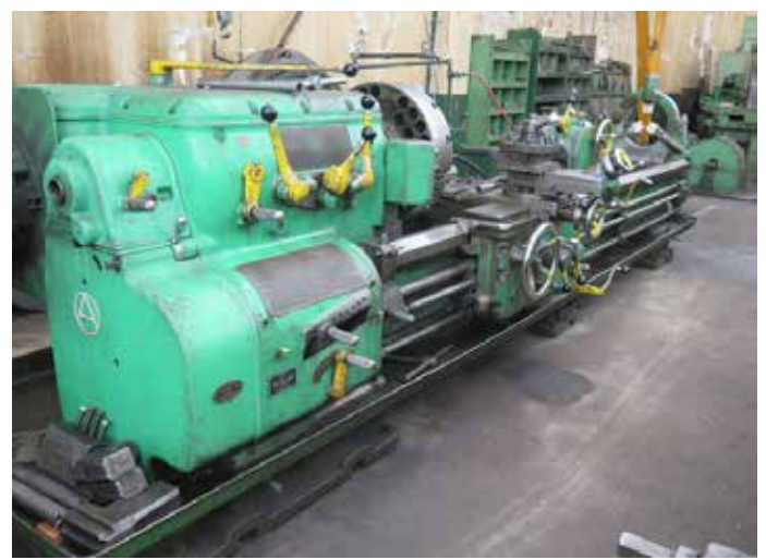
Axelson 25 25" x 192" Geared Head Lathe
