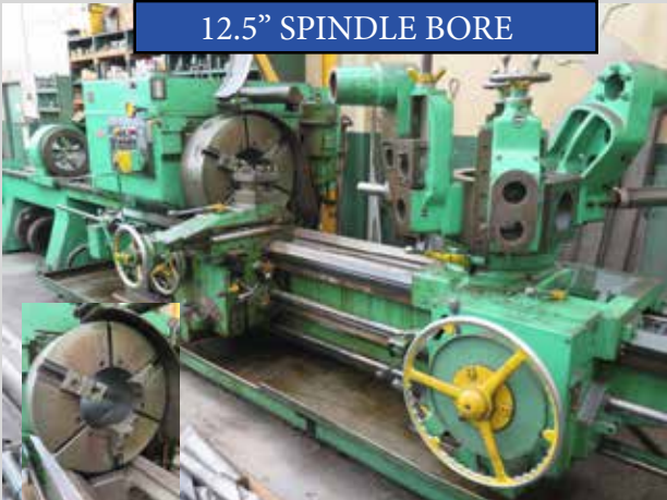
Warner & Swasey M-3580 Square Head Saddle Type Turret Lathe w/ 12 1/2" Thru Spindle Bore
