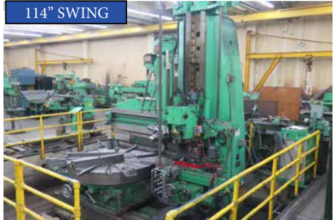
Berthiez type 9340/3 70" to 114" Open Side Vertical Boring Mill w/ Heidenhain DRO, 71" Table
