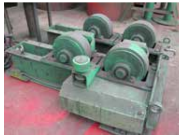
Aronson Motorized Tank Roll
