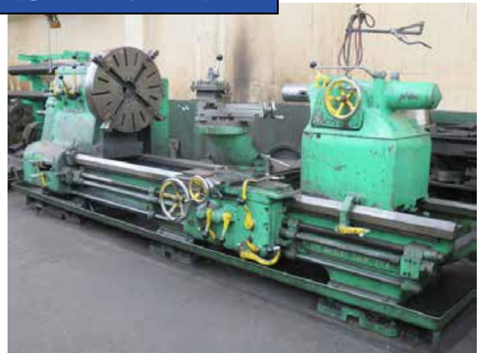
Axelson 32 (Factory Resized 14") 32" x 168" Engine Lathe w/ 59" Swing
