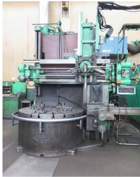
Bullard 61" Vertical Turret Lathe w/ 67" Swing
