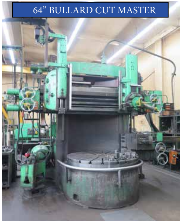
Bullard "Cut Master" 64" Vertical Turret Lathe w/ Miniwizard DRO, 69" Swing
