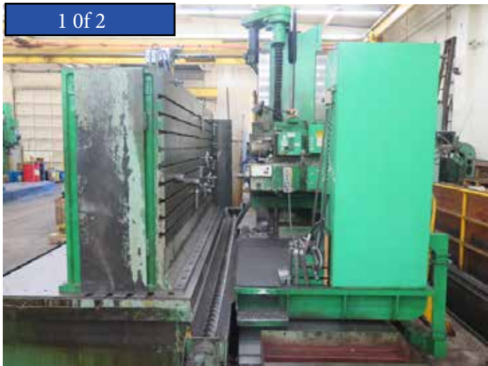
Cincinnati 48" x 168" CNC 3 Axis Traveling Column Horizontal HYDROTEL w/ AB 9/series CNC Controls
