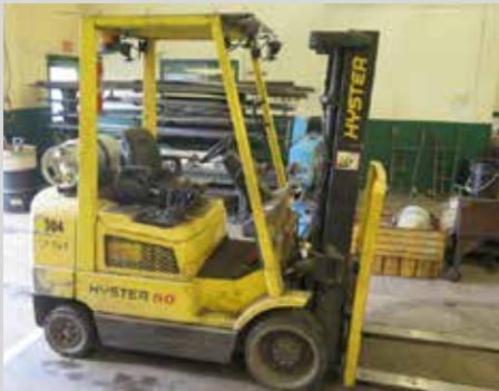
Hyster S50XM 5000 Lb Cap LPG Forklift
