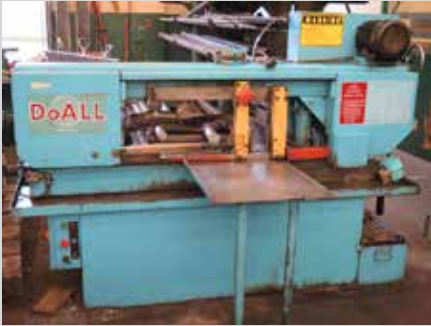
DoAll C-916M 9" Horizontal Band Saw
