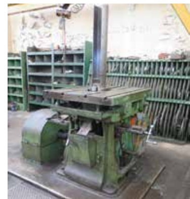
Mitts & Merrill No.6 Keyseater Machine
