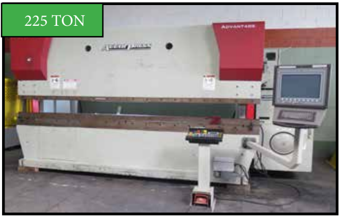
225 TON 2005 ACCURPRESS "ADVANTAGE 725012" 250 TON X 12' CNC HYDRAULIC PRESS BRAKE
