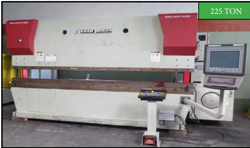
2005 ACCURPRESS "ADVANTAGE 725012" 250 TON X 12' CNC HYDRAULIC PRESS BRAKE S/N 3835 W/ ACCURPRESS ETS 3000 CONTROLS AND BACK GAUGING, ETS PEDESTAL CONTROLLER, 12' BED LENGTH, 10" THROAT DEPTH, 8" STROKE, 18" OPEN HEIGHT, 8" CLOSED HEIGHT, 125" BETWEEN UPRIGHTS, LIGHT CURTAIN
