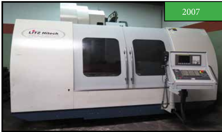
2007 LITZ HITECH CV-1400 CNC VERTICAL MACHINING CENTER W/ FANUC 01-MC CONTROLS, 24-STATION SIDE MOUNT ATC, 50 TAPER SPINDLE
