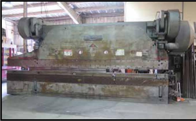
CINCINNATI 9-SERIES 225 TON X 17' MECHANICAL PRESS BRAKE W/ CINCINNATI AUTO CYCLE CONTROLS, PNEUMATIC CLUTCH
