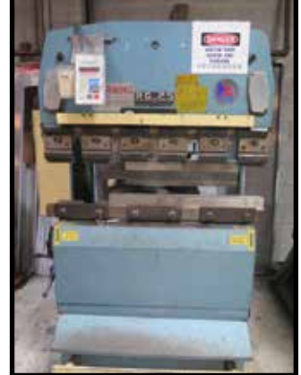
AMADA RG-25 25 TON X 48" CNC PRESS BRAKE W/AMADA "AUTOGAUGE" CNC CONTROLS
