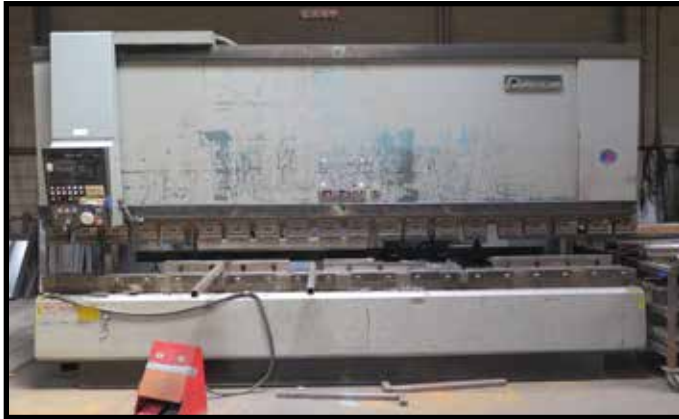
AMADA FCXB-200D 200 TON X 161" CNC PRESS BRAKE W/AMADA NC9-EX CONTROLS
