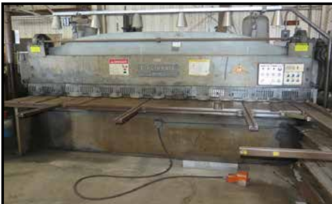
CINCINNATI 1812 1/2" X 12' HYDRAULIC POWER SHEAR W/ CINCINNATI "AUTO-SHEAR" 3-PROBE POWER BACK GAUGING SYSTEM
