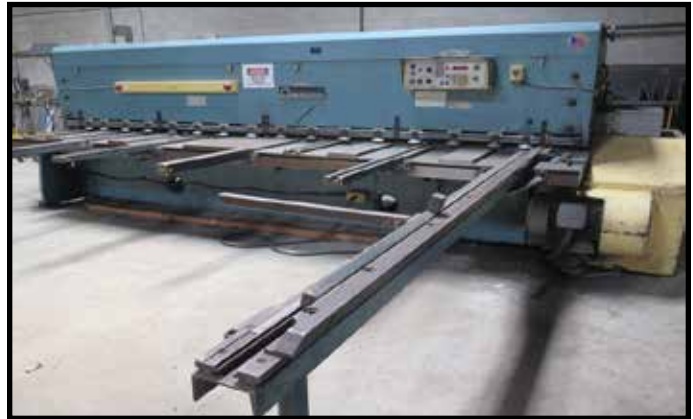
AMADA M-4065 4100MM(161.4") X 6.35MM(.25") CNC HYDRAULIC POWER SHEAR W/AMADA CONTROLS
