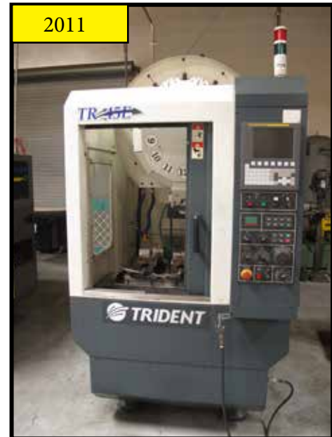
2011 TRIDET TR-45E CNC DRILL & TAP CENTER, FANUC OI-MD CONTROL, 12 ATC, 10,000 RPM, S/N 45E-11560.
