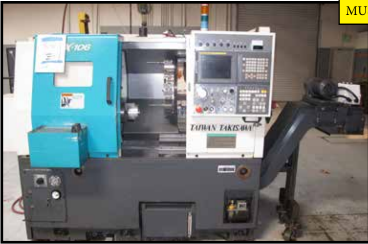
TAKISAWA EX-106 CNC LATHE, 6" CHUCK, 12 POSITION TURRET, FANUC 211-T CONTROL, CHIP CONVEYOR
