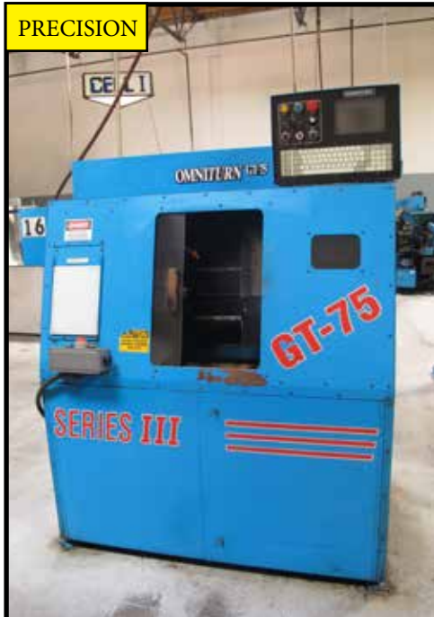
OMNI TURN GT75 CNC LATHE SERIES III, 12" X 9" TRAVELS, 4000 RPM, 5C, MODEL OT-CNC, S/N 392G34.
