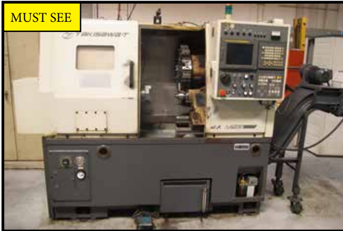
TAKISAWA EX-106 CNC LATHE WITH FANUC 211-TB CONTROL, 12 POS TURRET, TAIL STOCK, CHIP CONVEYOR, 6" CHUCK, EX SERIES.
