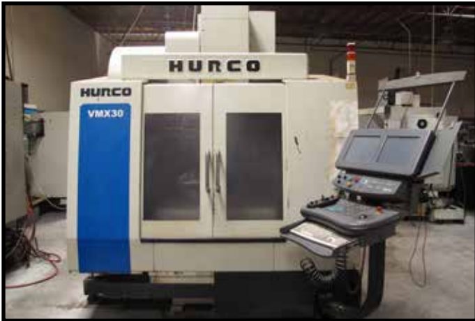
2005 HURCO VMX-30 CNC VMC, TRAVELS 30" X 20" X 24" (XYZ), 24 ATC, 40 TAPER, ULTIMAX CONTROL, S/N H-30549.
