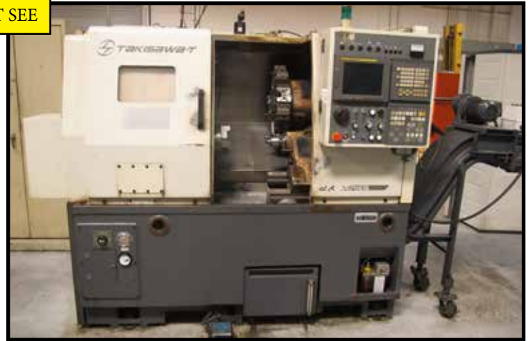
TAKISAWA EX-106 CNC LATHE WITH FANUC 211-TB CONTROL, 12 POS TURRET, TAIL STOCK, CHIP CONVEYOR, 6" CHUCK, EX SERIES.
