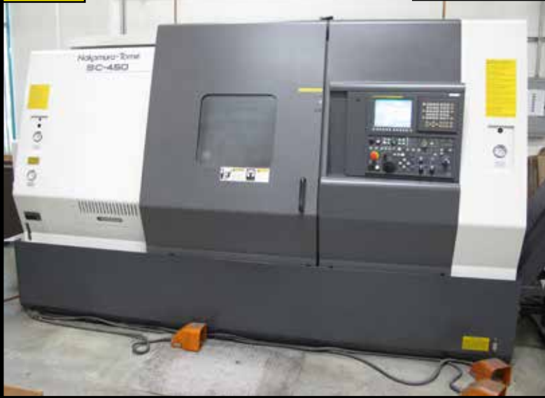
2013 NAKAMURA SC-450 CNC TURNING CENTER, 2 AXIS, 3.5' BAR CAPACITY 2500 RPM, WITH OPTIONAL 20" CHUCK, CHIP CONVEYOR, 12 POSITION TURRET, 28.14" MAX TURNING LENGTH, FANUC OI TD CONTROL, LOW HOURS, 40 HP, BOX WAYS, S/N S454403.
