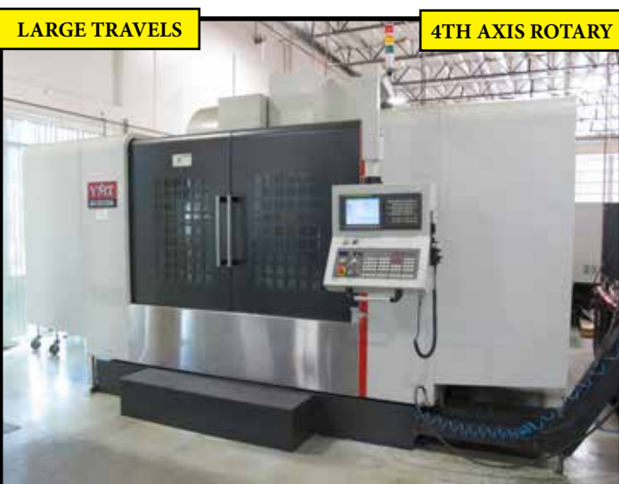
2012 YMT QV209A CNC VMC, 10,000 RPM, 40 TAPER, 30 ATC, FANUC OIMD, RIGID TAPPING, 78' X 35X33" (XYZ), S/N 1P011226K2.
