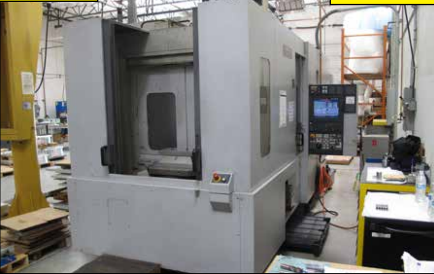
2004 MORI SEIKI NH 5000 CNC HMC, 12,000 PRM, BT-50, 120 ATC, S/N: NH501DH0658, FANUC MSX 501 (FANUC 18I MB) CONTROL, COOLJET CTS.
