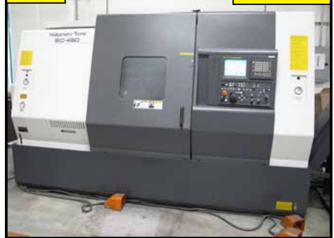
2013 NAKAMURA SC-450 CNC TURNING CENTER, 2 AXIS, 2500 RPM, WITH OPTIONAL 20" CHUCK, CHIP CONVEYOR, 12 POSITION TURRET, 28.14" MAX TURNING LENGTH, FANUC OI TD CONTROL, LOW HOURS, 40 HP, BOX WAYS, S/N S454403. 3.5" BAR CAPACITY
