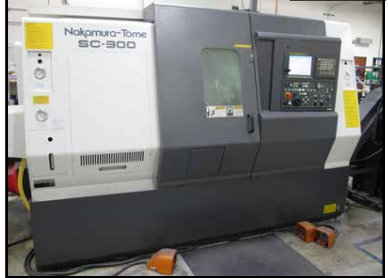
2014 NAKAMURA SC 300 CNC TURNING CENTER, 2 AXIS, 3500 RPM, WITH 12" CHUCK, CHIP CONVEYOR, 12 POSITION TURRET, 23.62" MAX TURNING LENGTH, 2.5' BAR CAPACITY FANUC OI TD CONTROL, 30 HP, S/N S312201.
