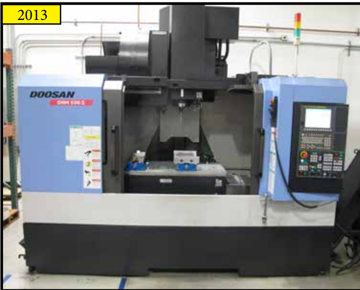
2013 DOOSAN 500 II CNC VMC, 12,000 RPM, 30 ATC, 40 TAPER, 40.2" X 21.3" X 20.1" (X Y Z), RIGID TAPPING, RENISHAW PROBING, FANUC SERIES 1, 4 TH AXIS DRIVE, S/N MV0010-002320.
