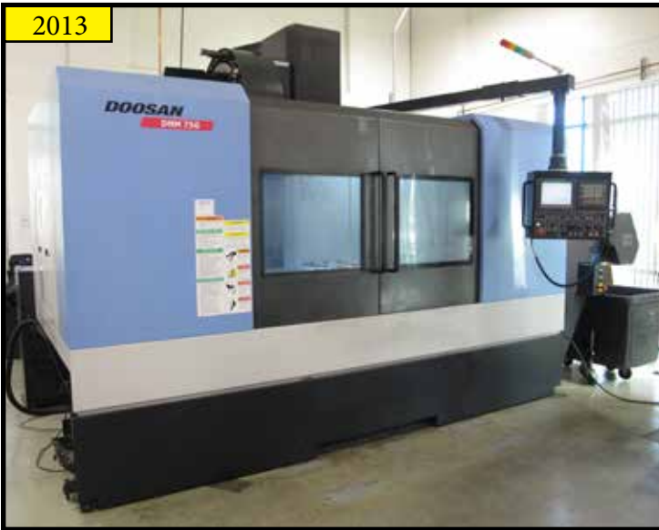
2013 DOOSAN DNM-750 II CNC VMC, 12,000 RPM, 30 ATC, 40 TAPER, FANUC SERIES 1,, 64" X 30" X 25.6" (X Y Z), RIGID TAPPING, RENISHAW PROBING, 4 TH AXIS DRIVE, S/N MV0064-000070.
