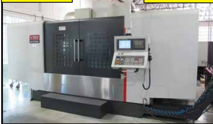
2012 YMT QV209A CNC VMC, 10,000 RPM, 40 TAPER, 30 ATC, FANUC OIMD CONTROL, RIGID TAPPING, 78" X 35" X 33" (X Y Z), S/N 1P011226K2.
