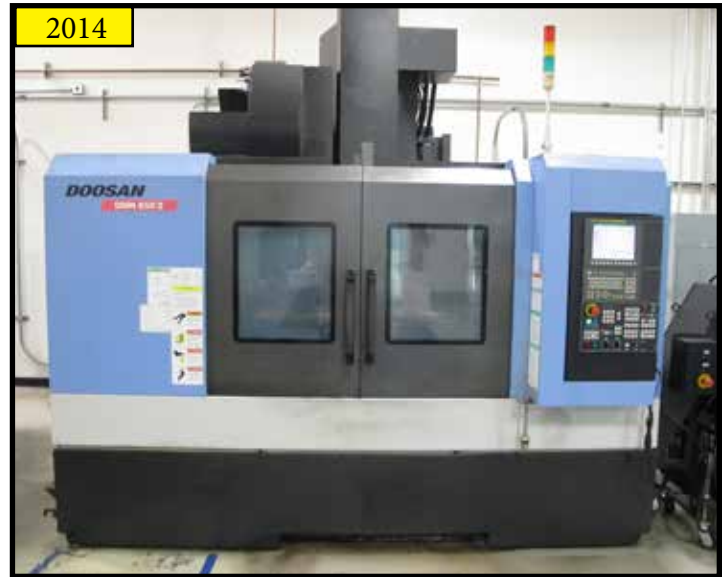
2014 DOOSAN 650 II CNC VMC, 12,000 RPM, 30 ATC, 40 TAPER, 50" X 26.4" X 24.6" (X Y Z), RIGID TAPPING, RENISHAW PROBING, FANUC SERIES 1, 4 TH AXIS DRIVE, S/N MV0011-001482.
