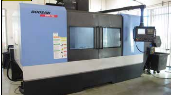
2013 DOOSAN DNM-750 II CNC VMC, 12,000 RPM, 30 ATC, 40 TAPER, FANUC SERIES 1, 64" X 30" X 25.6" (X Y Z), RIGID TAPPING, RENISHAW PROBING, 4 TH AXIS DRIVE, S/N MV0064-000070.
