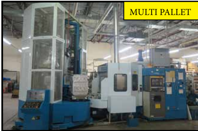
Toyoda FH55 4-Axis Multi Pallet CNC Horizontal Machining Center w/ Fanuc 11M Controls, 120-ATC, CAT-50 Spindle, 12-Pallet Vertical Pallet Changer System
