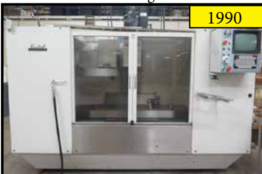
1990 Fadal VMC4020 CNC Vertical Machining Center w/ CNC88 Controls, 21-ATC, CAT-40 Spindle
