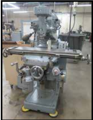
Tree 2VGC Vertical Mill w/ 3Hp Motor, Colleted Spindle, Box Ways, Power "X" and Knee Feeds
