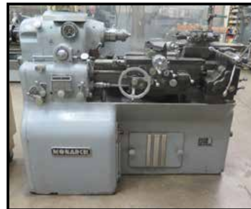
Monarch 10"EE 12 1/2" x 20" Lathe w/ 0-3000 RPM, 6-Station Turret, 5C Collet Closer
