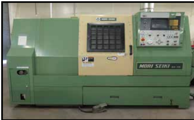
Mori Seiki SL-15 CNC Turning Center w/ Fanuc 10T Controls, Tool Presetter
