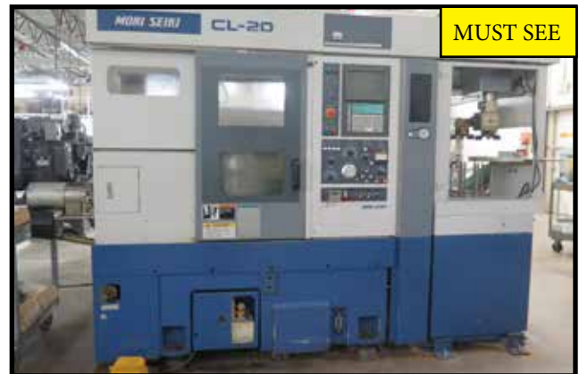
Mori Seiki CL-20A CNC Turning Center w/ Yasnac Controls, Mori Seiki Robotic Gantry Parts Loader /Unloader
