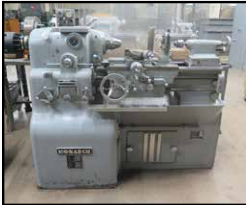
Monarch 10"EE 12 1/2" x 20" Lathe w/ 0-3000 RPM, Pneumatic 5C Collet Closer
