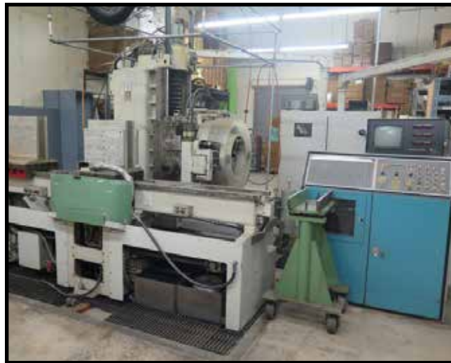
Kearney & Trecker Milwaukee-Matic / KTNC Multi Pallet NC Sliding Column Horizontal Boring Mill
