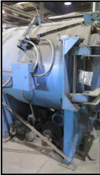
Lindburg Isobrite type 0921830124CX 1400 Deg F Vacuum Furnace
