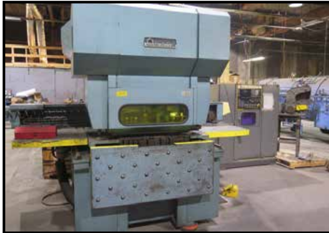
Amada OCTO 30-30-40 30-Ton 8-Station CNC Inline Punch Press w/ Amada-Fanuc-0 System 6M Controls
