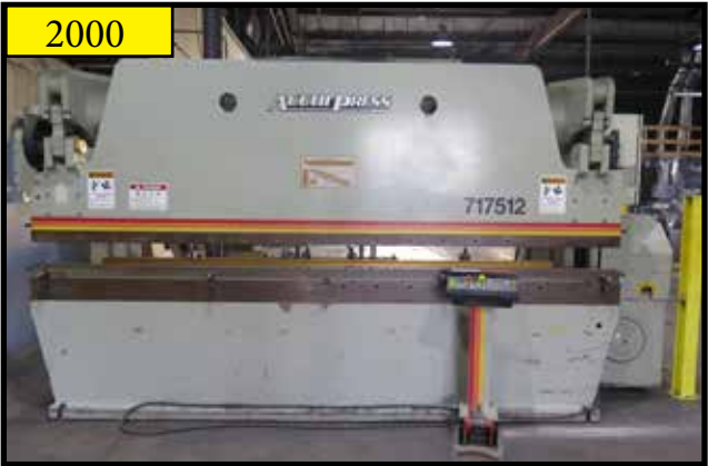
2000 Accurpress 717512 175 Ton x 12' CNC Hydraulic Press Brake
