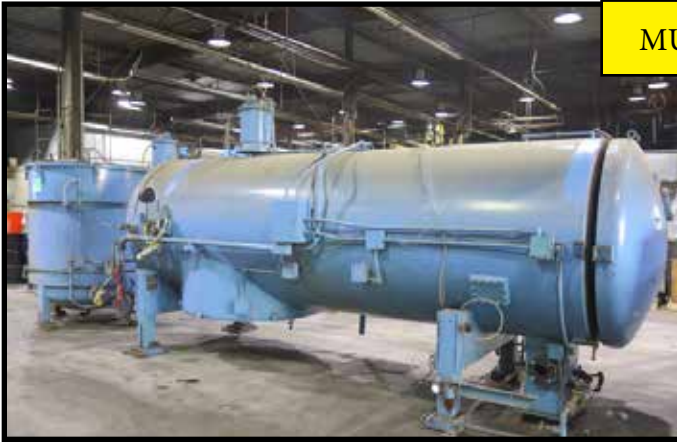
Lindburg Isovac type 09318-30124BRSX 2400 Degree F Vacuum Furnace
