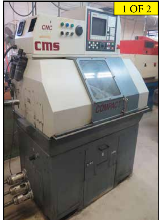
CMS "Compact GT-27" CNC Cross Slide Lathe w/ Fagor 8050/55-T Controls
