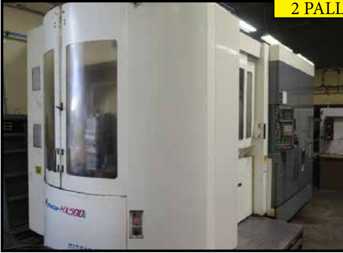
Kitamura Mycenter-HX500i 2-Pallet 4-Axis CNC Horizontal Machining Center w/ Fanuc 16i-M Controls, 50-ATC, CAT-50, 12,000 RPM
