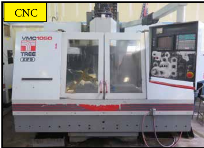
Tree ZPS VMC-1050/24 CNC Vertical Machining Center w/ Yasnac Controls, 24-ATC
