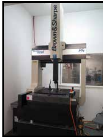
Brown & Sharpe "Micro Xcel PFx" CMM Machine w/ Renishaw PH10MG Motorized Probe
