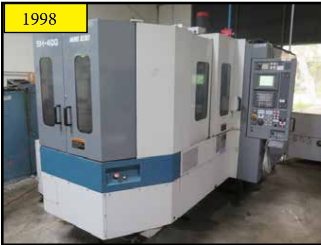
1998 Mori Seiki SH-400 2-Pallet 4-Axis CNC Horizontal Machining Center w/ MSC-518 Controls, 40-ATC, CAT-40, 12,000 RPM
