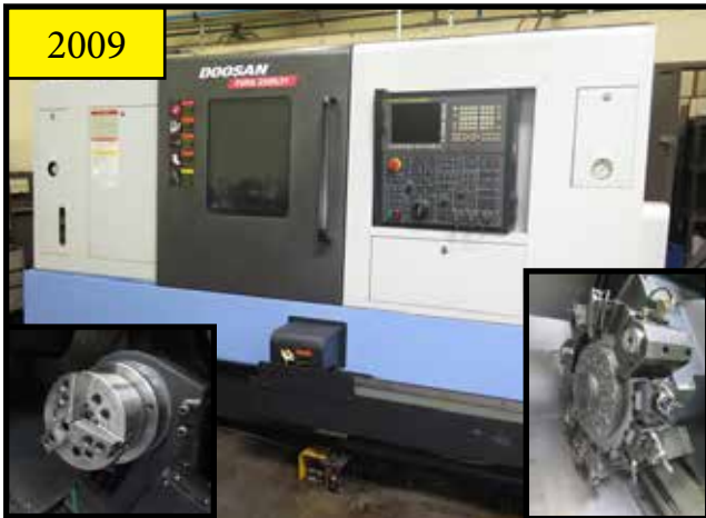
2009 Doosan PUMA 2500LSY Twin Spindle Live Turret CNC Turning Center w/ Fanuc 31i-Model A Controls, Tool Presetter, 12/24 Station Fully Live Turret
