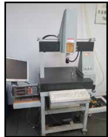
Numerex 1312-10 CMM Machine w/ Micron-X 3-Axis DRO
