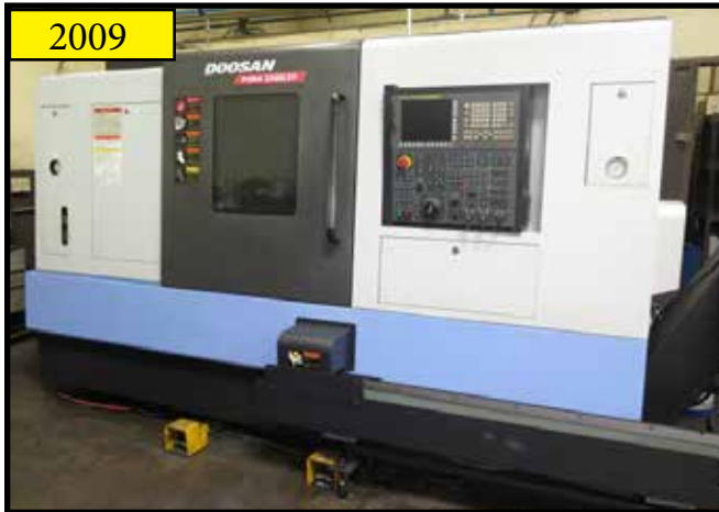
2009 Doosan PUMA 2500LSY Twin Spindle Live Turret CNC Turning Center w/ Fanuc 31i-Model A Controls, Tool Presetter, 12/24 Station Fully Live Turret
