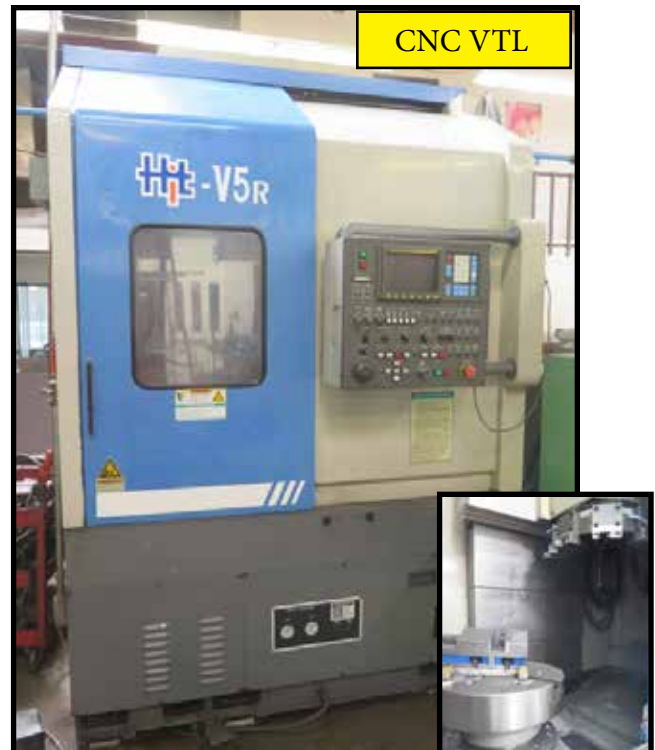
Hyundai HiT-V5R CNC Vertical Turret Lathe w/ Fanuc 0-T Controls, 8-Station Turret, 2500 RPM, 21"3-Jaw Power Chuck
