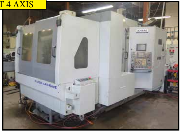
Hyundai KH50G 2-Pallet 4-Axis CNC Horizontal Machining Center w/ Fanuc 18i-MB Controls, Renishaw Non-Contact Tool Presetter, 60-ATC, CAT-5
