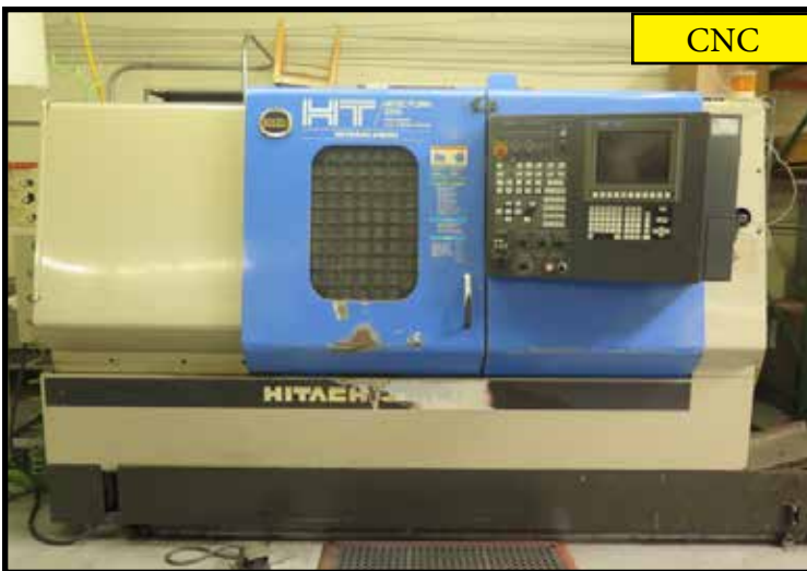
Hitachi Seiki HITEC-TURN 25G High Grade CNC Turning Center w/ Hitachi Seiki Seicos Delta 10L Control
