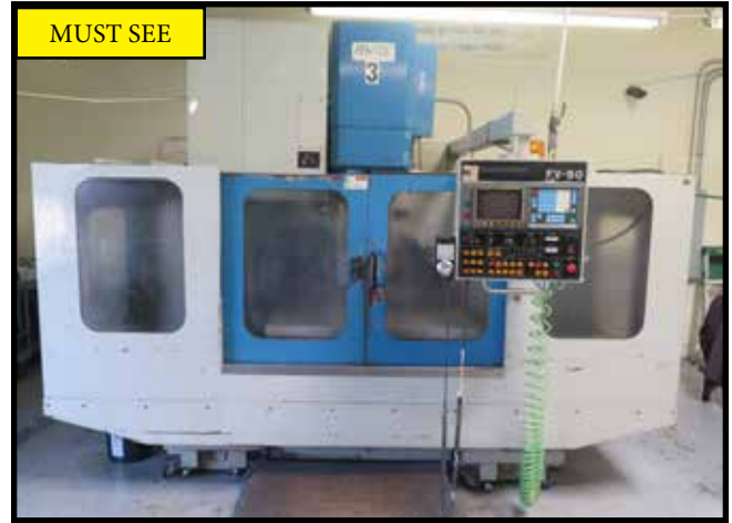
1998 Femtec / Kafo FV-50 CNC Vertical Machining Center w/ Fanuc 0-M Controls, 24-Station Side Mount ATC, CAT-50 Spindle
