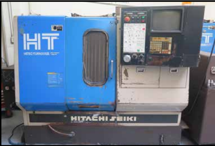
Hitachi Seiki HITEC-TURN 20 SII Super Productive Turning Cell w/ Hitachi Seiki Controls, Tool Presetter
