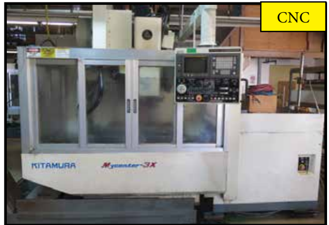
Kitamura Mycenter-3X 2-Pallet CNC Vertical Machining Center w/ Fanuc 0-M Controls, 24-Station ATC, CAT-40 Spindle, 10,000 RPM
