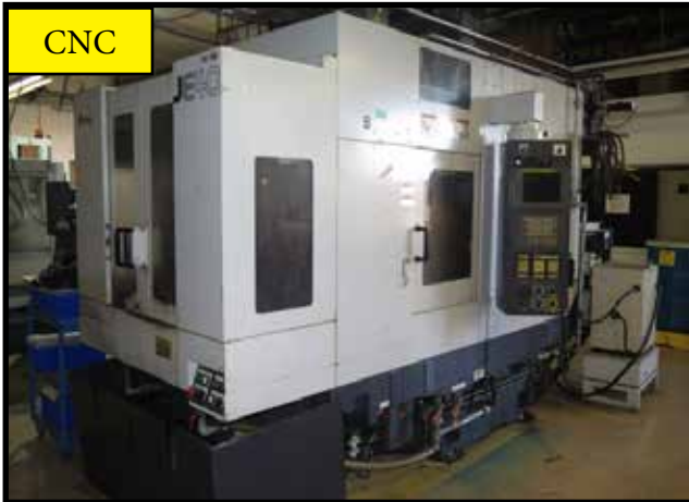
Enshu JE-40 2-Pallet 4-Axis CNC Horizontal Machining Center w/ Fanuc 18i-M Controls, 30-Station ATC, CAT-40 Spindle
