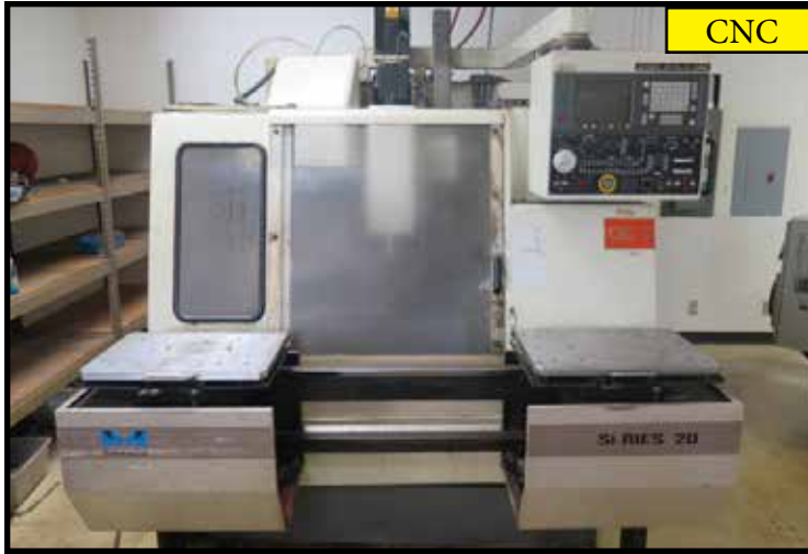
Kitamura Mycenter-1/485 2-Pallet CNC Vertical Machining Center w/ Fanuc Controls, 16-Station ATC, BT-35 Spindle, Midaco Shuttle System
