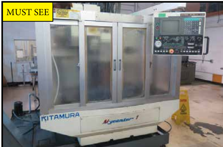
Kitamura Mycenter-1 CNC Vertical Machining Center w/ Yasnac Controls, 20-Station ATC, BT-40 Spindle, 13,000 RPM
