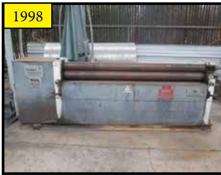
1998 Famar / Eagle A3122012 74" Power Pinch Roll
