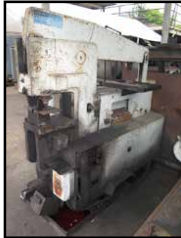
Scotchman / Excel mdl. 7012 70 Ton Hydraulic Iron Worker
