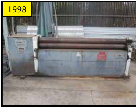
1998 Famar / Eagle A3122012 74" Power Pinch Roll
