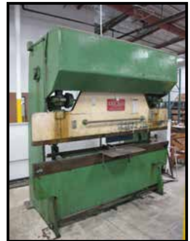
CHICAGO MODEL 68-B, 8FT X 55 TON MECHANICAL PRESS BRAKE.
