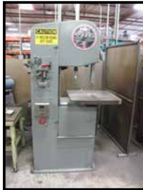
DO ALL DBW-15, 15" VERTICAL BAND SAW WITH WELDER.
