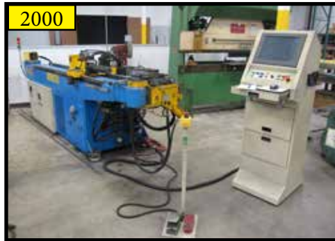
2000 CSM CNC TUBE BENDER, MODEL C38TSR, 3 AXIS 3M CONTROL, 1.5" CAP,MANDRAL TYPE.
