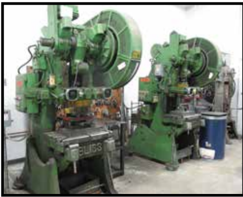
2) BLISS MODEL 21B 50 TON MECHANICAL PUNCH PRESS, PALM BUTTONS, AIR CLUTCH.
