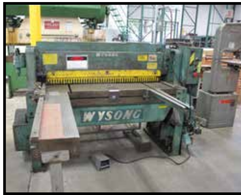
WYSONG 1052, 52" X 10GA MECHANICAL POWER SHEAR W/ SQUARING ARM
