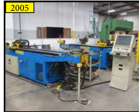
2005 CSM CNC TUBE BENDER, MODEL C38TSR, 3 AXIS 3M CONTROL, 1.5" CAP,
