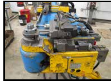
2000 CSM CNC TUBE BENDER, MODEL C38TSR, 3 AXIS 3M CONTROL, 1.5" CAP,MANDRAL TYPE.
