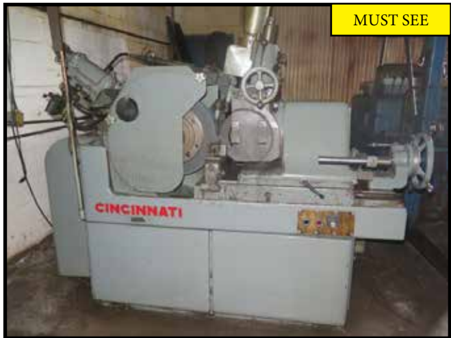
Cincinnati OM Centerless Grinder w/ AC Regulating Wheel Drive Conversion, 24" Grinding Wheel
