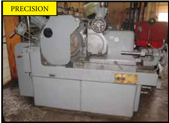
Cincinnati OM Centerless Grinder w/ 24" Grinding Wheel
