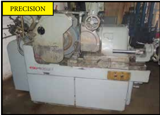
Cincinnati OM Centerless Grinder w/ 24" Grinding Wheel
