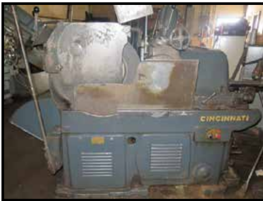
Cincinnati EA Centerless Grinder w/ OM Taper Screw Conversion, 20" Grinding Wheel
