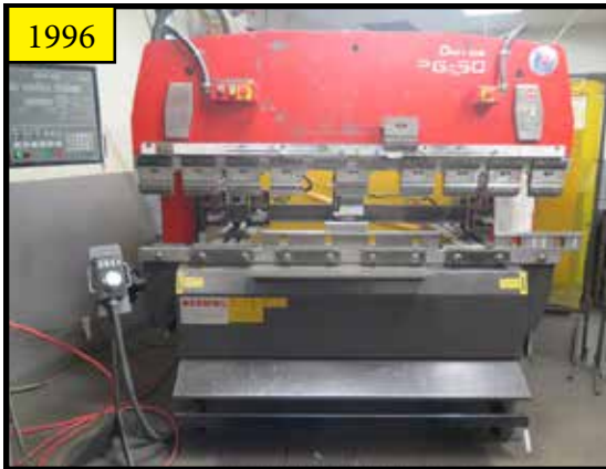
1996 Amada RG-50 50-Ton x 82" CNC Press Brake w/ Amada NC9-EX II Controls
