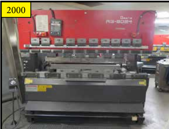
2000 Amada RG-8024 LD 80-Ton x 98" CNC Press Brake w/ Amada LD Controls
