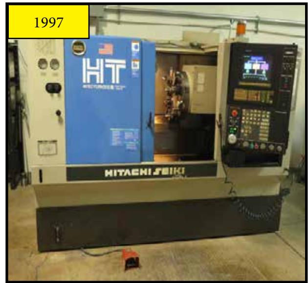
1997 Hitachi Seiki, HT Hitec-Turn 20S III / Super Production Turning Cell, DS3006HL Hitachi Seiki Control, 10 Tool Turret, Programmable Tail Stock.
