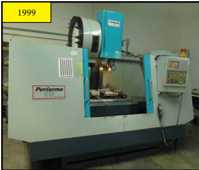
V5 1999 Akira-Seiki, Preforma V5 Vertical Machining Center, Mitsubishi Control, 99VNCNO30-15B 51" x 22" Travels, 8000 RPM, 24 ol Swing Arm ATC
