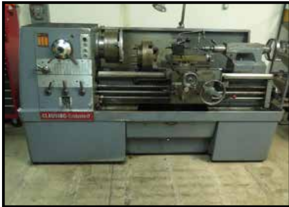
Clausing Colchester, Gap Bed Lathe, 17" Swing, 60" Centers, 5C Lever 80 52 7001402899 Action Collet Closer, 12" 3 Jaw Chuck, Quick Change Tooling, Travidial.
