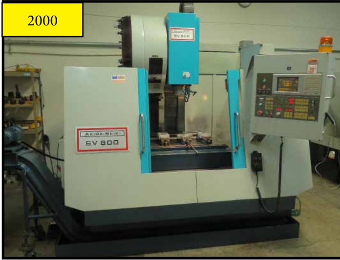
2000 SV800 2000 Akira-Seiki, SV-800 Vertical Machining Center, Mitsubishi Control, OOVG840-306 32" x 19" Travels, 10,000 RPM, Swing Arm ATC,
