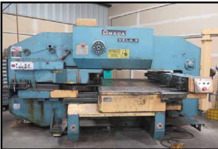
Amada VELA II 305050 30 Ton CNC Turret Punch Press w/ Amada-Fanuc-V Controls
