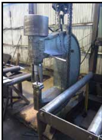
Whitney 791-0001 90 Ton C-Frame Beam Punch w/ 13" Throat
