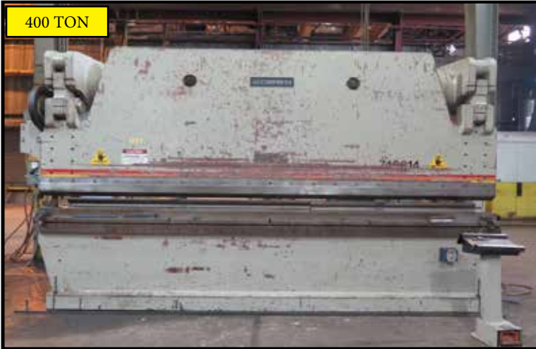
1998 Accurpress 740014 400 Ton x 14' CNC Hydraulic Press Brake
