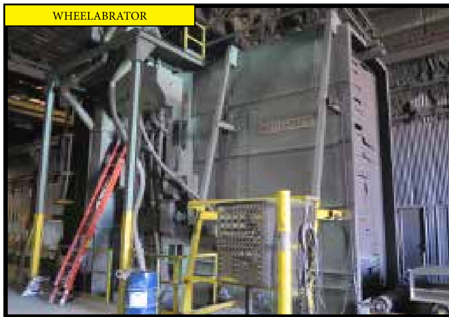
Wheelabrator Pass-Thru Blast Booth w/ Wheelabrator Controls, (8) 25Hp Blast Heads, 6' x 9' Capacity
