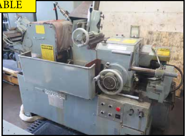
Cincinnati Milacron "CINCO-15" mdl. DR Centerless Grinder w/ 24" Grinding Wheel
