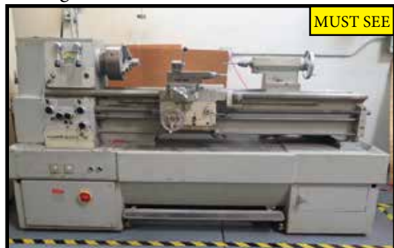
Harrison 15" 15" x 55" Geared Head Gap Bed Lathe
