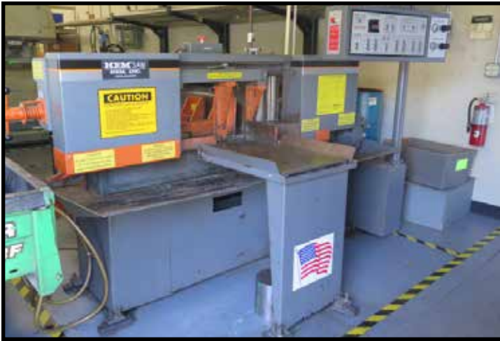
HEM H90A-4 12" Automatic Horizontal Band Saw
