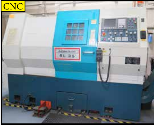
Akira Seiki SL-35 CNC Turning Center w/ Fanuc Oi-TC Controls
