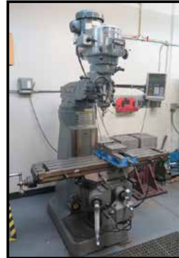
Bridgeport - Hardinge Vertical Mill w/ Newall C80 DRO
