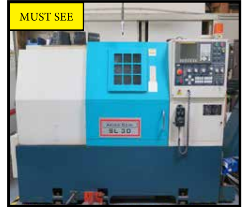
Akira Seiki SL-30 CNC Turning Center w/ Fanuc Oi-TC Controls
