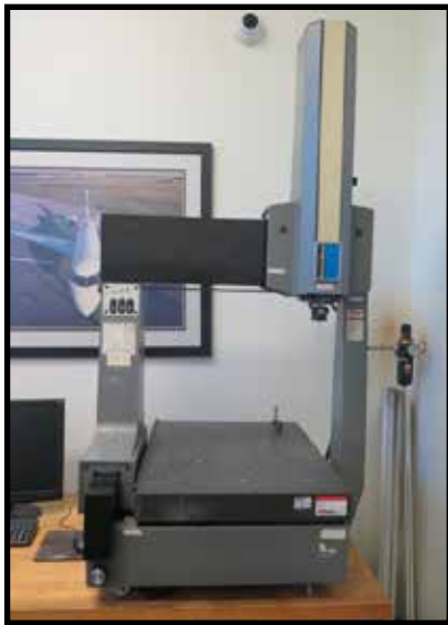
Brown & Sharpe CMM Machine w/ Renishaw TP1S Probe
