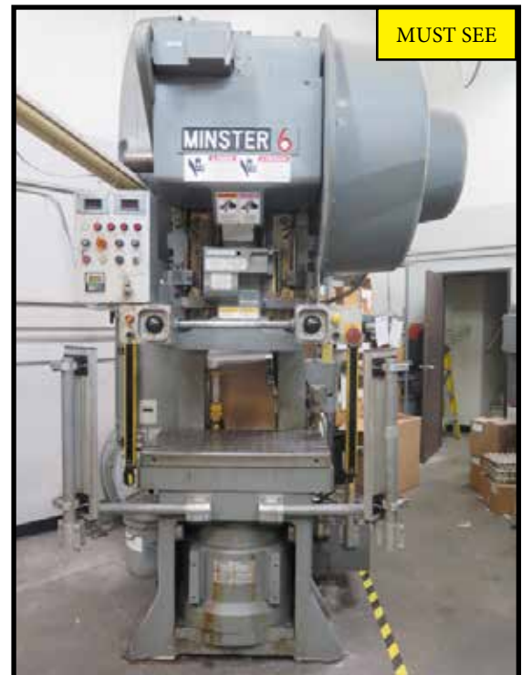
Minster 6 60 Ton OBS Fixed Base Stamping Press w/ Minster Controls, 45-90 Strokes/Min
