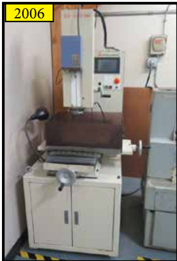
2006 Mitsubishi / Mikuni Makino ED-2000M Small-Hole Drilling EDM Machine
