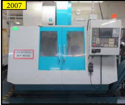
2007 Akira Seiki SC-800 CNC Vertical Machining Center w/ Mitsubishi Controls
