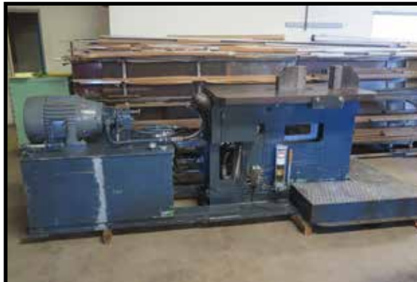
J.A. Richards "Multiform Bender" 3/8" x 8" Horizontal Hydraulic Bending Machine
