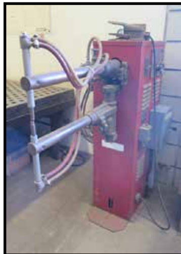
Western Arctronics Type 15-SA 15kVA Spot Welder
