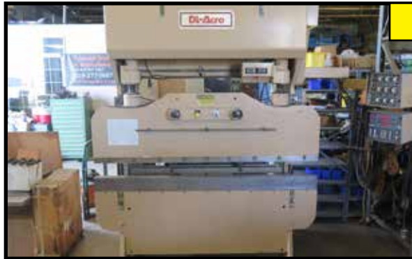
DiAcro 75-6 75 Ton x 6" CNC Hydra-Power Press Brake w/ Dynabend I Controls
