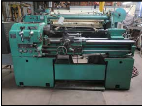
Homach KM-1800 15" x 52" Geared Head Gap Bed Lathe
