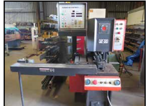
Amada SP-30 30 Ton Hydraulic Press w/ Amadan-SS Controls
