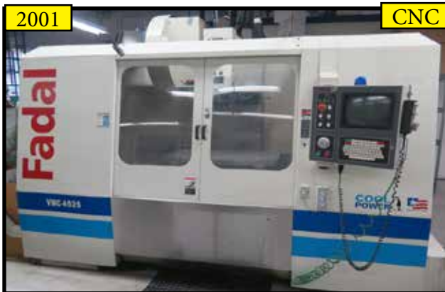
2001 Fadal VMC4524 4-Axis CNC Vertical Machining Center w/ Multi Processor CNC Controls, 24-Station Side Mount ATC, BT-40 Spindle, 10,000 RPM, Rigid Tapping
