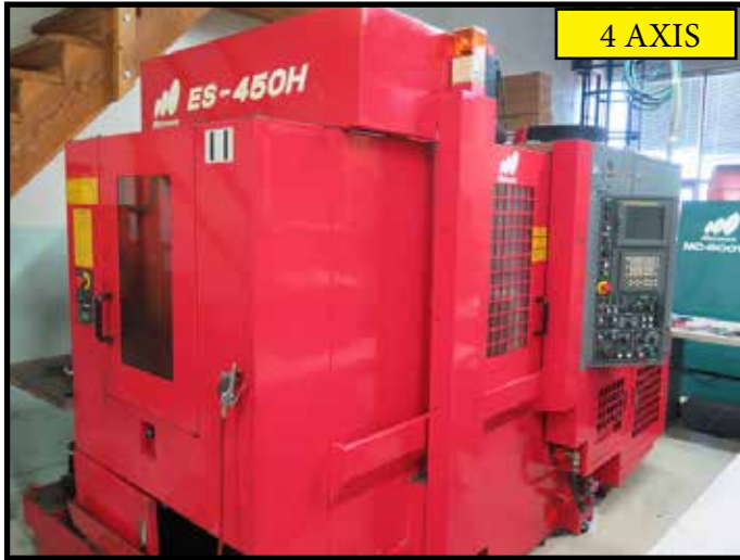
1998 Matsuura ES-450H 2-Pallet 4-Axis CNC Horizontal Machining Center w/ Fanuc 18i-M Controls, 30-ATC, BT-40 Spindle, 10,000 RPM, NEW SPINDLE, Tool Presetter
