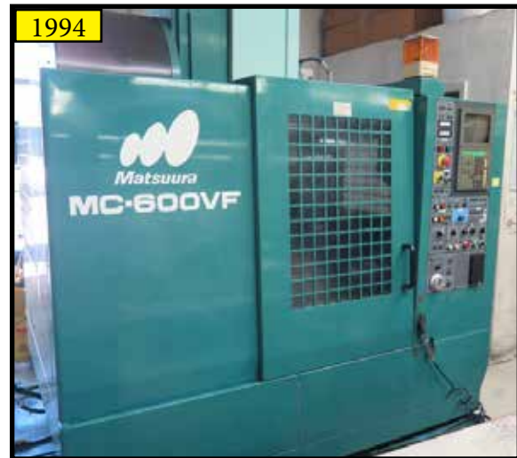
1994 Matsuura MC-600VF CNC Vertical Machining Center w/ Yasnac i-80 Controls, 20-ATC, BT-40 Spindle, 8000 RPM
