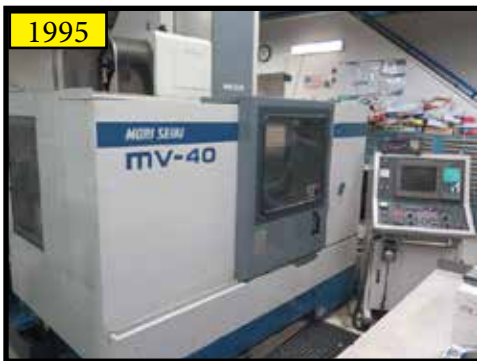
1995 Mori Seiki MV-40/40 CNC Vertical Machining Center w/ Yasnac Control Console, 20-ATC, BT-40 Spindle, 8000 RPM
