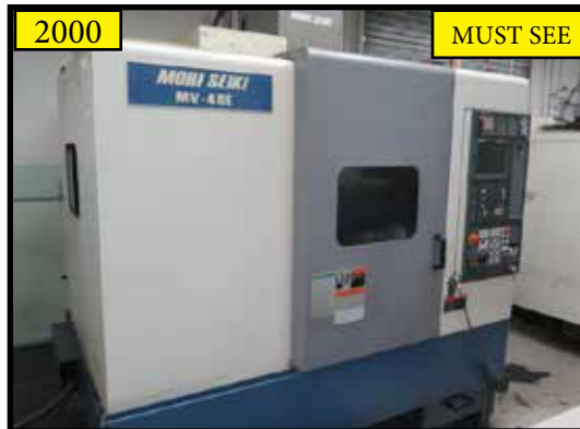
2000 Mori Seiki MV-40E 4-Axis CNC Vertical Machining Center w/ MSC-500 Controls, 20-ATC, BT-40 Spindle, 10,000 RPM
