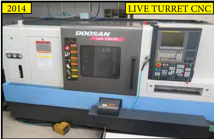
2014 Doosan LYNX 220 LMSA Twin Spindle Live Turret CNC Turning Center w/ Doosan Fanuc i-Series Controls, Tool Presetter, 12/24 Station Live Turret, 12-Live Stations, 6000 RPM Main, Sub and Rotary Spindles, "C" Axis Rotation @ 0.001 Degrees
