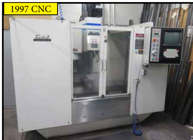
1997 Fadal VMC 3016HT CNC Vertical Machining Center w/ CNC88HS Controls, 21-ATC, CAT 40 Spindle, 10,000 RPM
