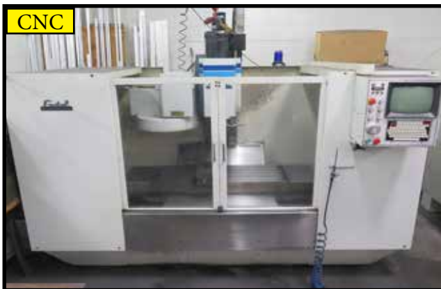
Fadal VMC 4020 CNC Vertical Machining Center w/ CNC88 Controls, 21-ATC, CAT-40 Spindle, 10,000 RPM
