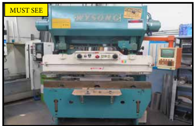
MUST SEE Wysong H-60- 72 60-Ton x 72" CNC Press Brake w/ Dynabend III Controls
