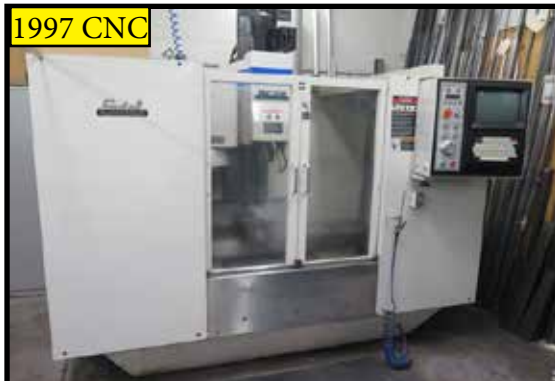
1997 Fadal VMC 3016HT CNC Vertical Machining Center w/ CNC88HS Controls, 21-ATC, CAT 40Spindle, 10,000 RPM
