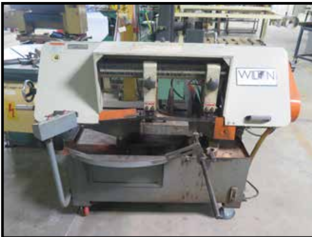
Wilton 7020M 11" Horizontal Mite Band Saw
