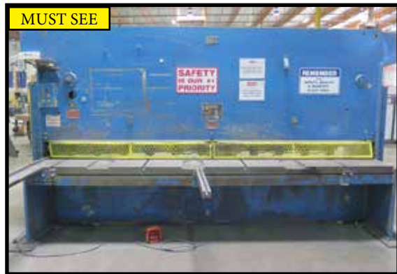
HTC 250-12A 1/4"/10GA x 12' Hydraulic Power Shear
