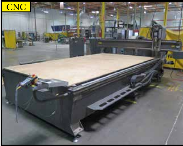
MultiCam 5000 Series CNC Router w/ HMI 20 Pendant Control, 12-Station ATC
