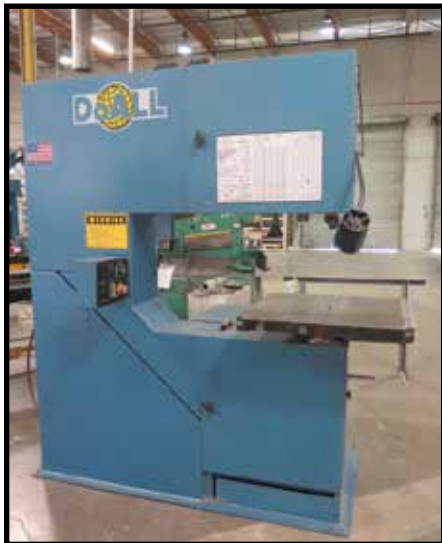
DoAll mdl. 3613-V3 36" Vertical Band Saw
