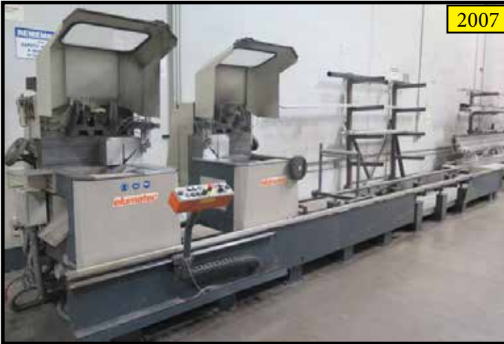
2007 Elumatec Type DG142/02 Double Up-Acting Miter Saw
