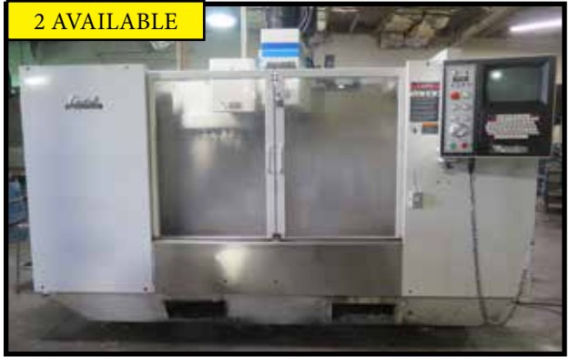
1997 Fadal VMC 4020 CNC Vertical Machining Center w/ CNC88HS Controls, 21-ATC, CAT-40Spindle, 28" Extended "Z" Axis
