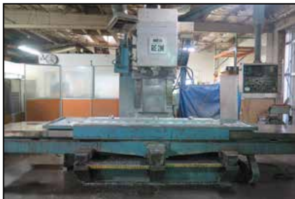
OOYA RE-2M CNC Vertical Machining Center w/ GN-Fanuc 6 Series Controls, 32-ATC, CAT-50 Spindle
