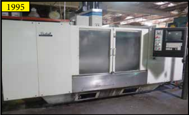
1995 Fadal VMC 6030HT CNC Vertical Machining Center w/ CNC32MP Controls, 21-ATC, CAT-40Spindle
