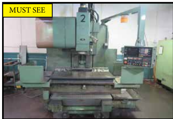
MUST SEE Enshu VMC 610 CNC Vertical Machining Center w/ Fanuc 6M Controls, 30-ATC, CAT-50 Spindle
