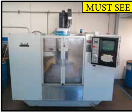
1996 Fadal VMC2216HT CNC Vertical Machining Center w/ Fadal CNC88HS Controls, 21-ATC, CAT-40 Spindle, 10,000 RPM
