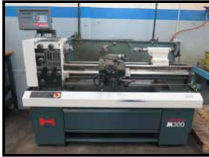
Harrison M300 13" x 42" Geared Head Lathe w/ Newall DP7 Programmable DRO
