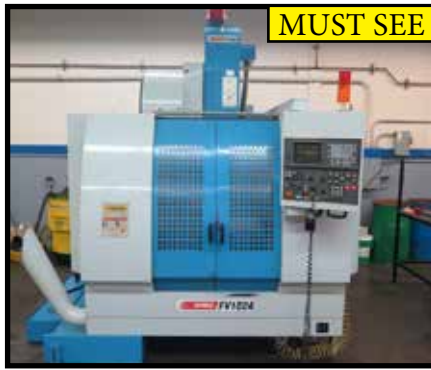
Supermax FV102A CNC Vertical Machining Center w/ Fanuc 18-M Controls, 24-ATC, CAT-40 Spindle, 10,000 RPM
