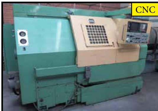
Hitachi Seiki NF20 Twin Turret CNC Turning Cell w/ Fanuc 6T Controls
