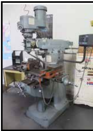
Bridgeport Series 1 - 2Hp Vertical Mill w/ Mitutoyo KA Counter DRO
