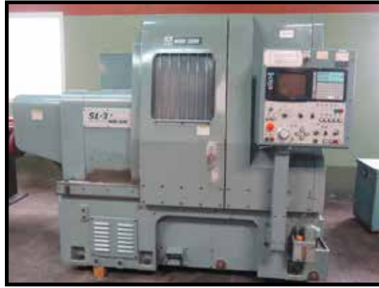
Mori Seiki SL-3H CNC Turning Center w/ Yasnac Controls
