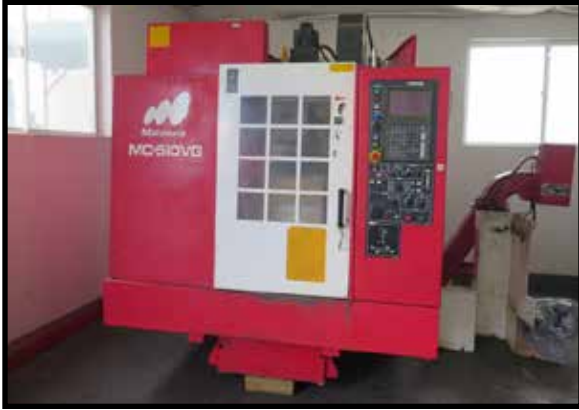
1998 Matsuura MC510VG CNC Vertical Machining Center w/ Yasnac Controls
