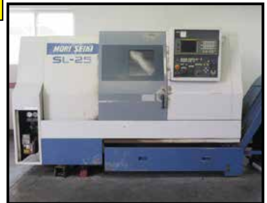
Mori Seiki SL-25B CNC Turning Center w/ Fancu MF-T6 Controls
