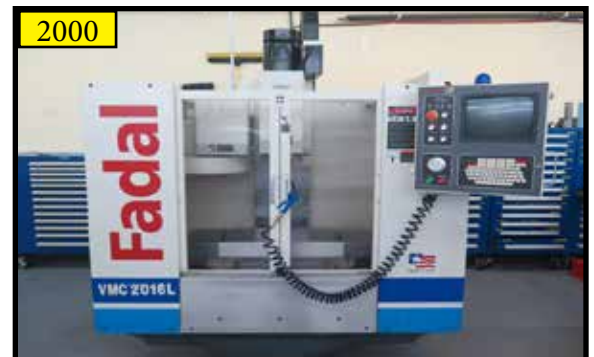
2000 Fadal VMC2016L CNC Vertical Machining Center w/ Fadal Multiprocessor Controls, 21-ATC, AT-40 Spindle
