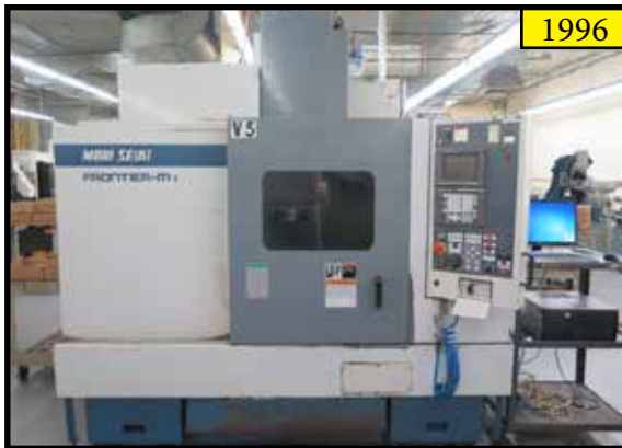
1996 Mori Seiki Frontier-M II CNC Vertical Machining Center w/ MSC-521 Controls, 20-Station ATC, CAT-40 Spindle
