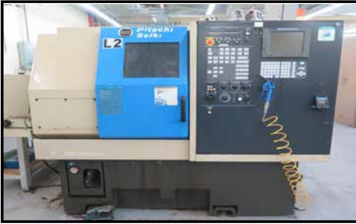
2000 Hitachi Seiki TS15 CNC Turning Center w/ Hitachi Seiki Controls, Tool Presetter, 12-Station Turret
