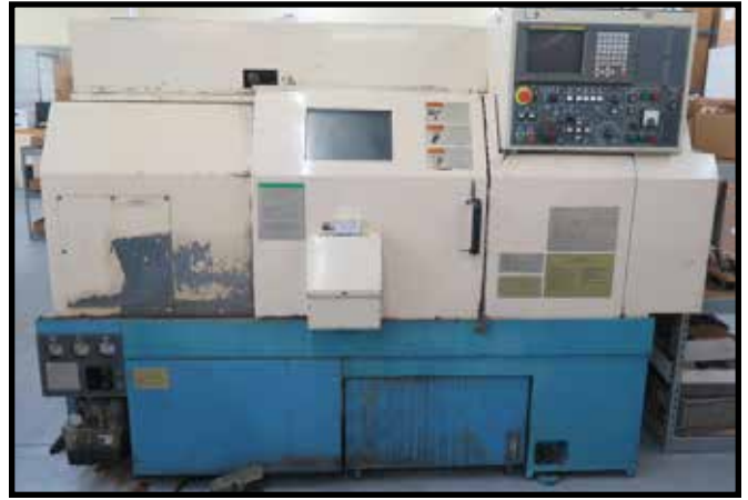
1996 Dianichi F-20 CNC Turning Center w/ Fanuc 18-T Controls, Tool Presetter, 12-Station Turret
