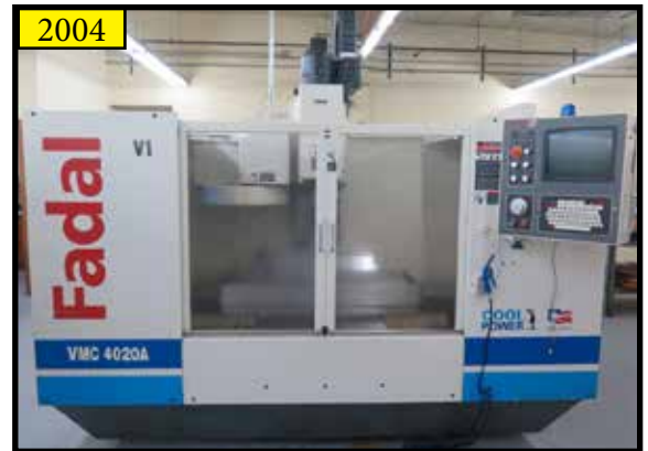
2004 Fadal VMC4020AHT CNC Vertical Machining Center w/ Fadal Multiprocessor Controls, 21-ATC, CAT-40 Spindle
