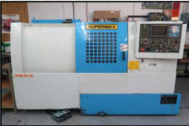
Supermax YCM-TC- 15 CNC Turning Center w/ Fanuc Series 0-T Control
