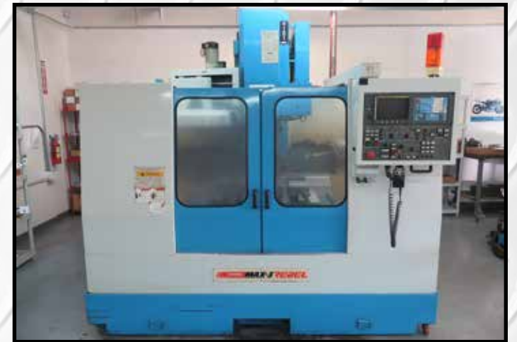
1999 Supermax MAX-3 Rebel CNC Vertical Machining Center w/ Fanuc 0-M Control
