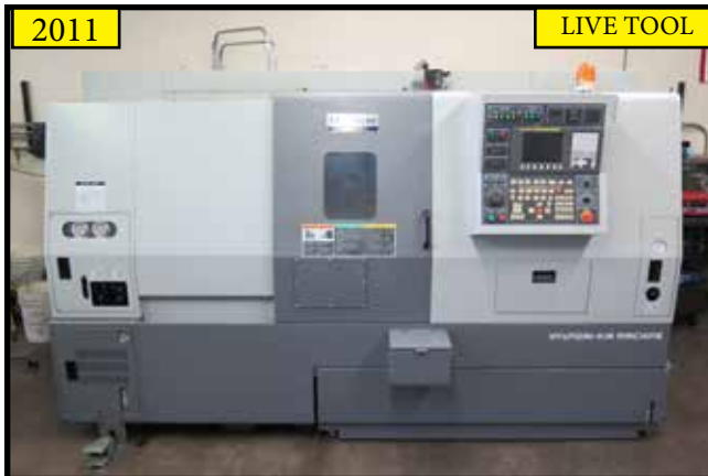
2011 Hyundai - KIA KT15 LMS Sub Spindle, Live Turret CNC Turning Center w/ Fanuc 0i-TC Controls
