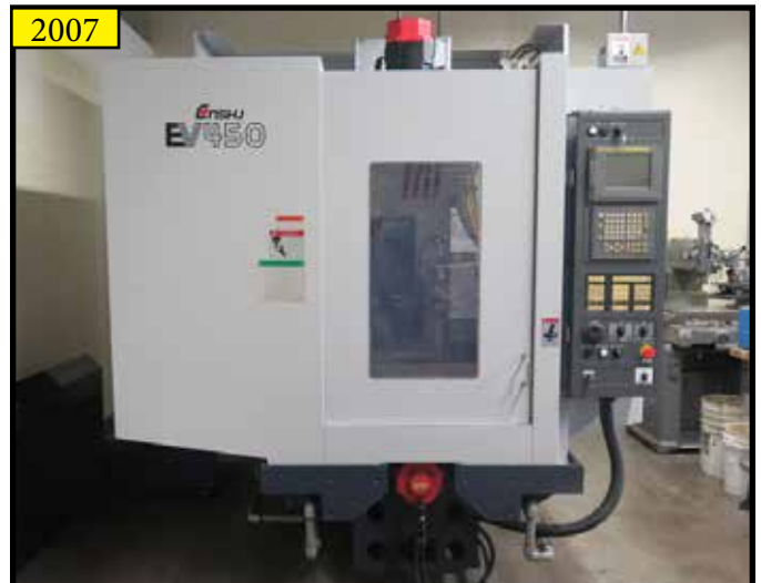
2007 Enshu EV450 CNC Vertical Machining Center s/n 402 w/ Fanuc Series 18i-MB Controls
