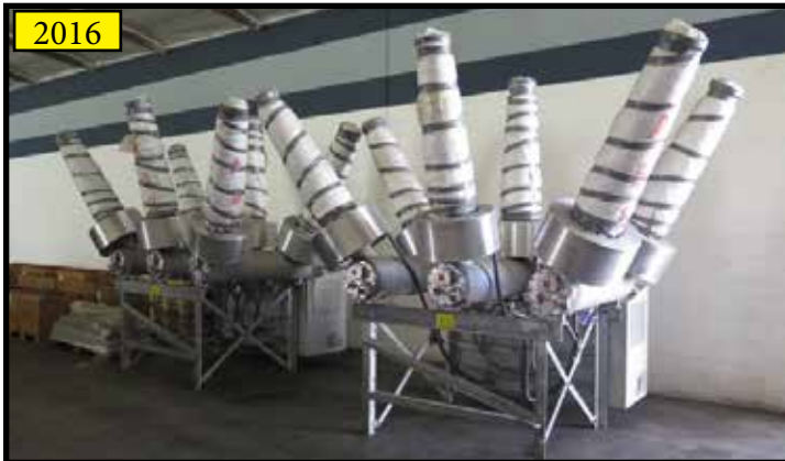
2016 ABB Type 145PM40-12C “SF6 Power Circuit Breaker” 145kV
