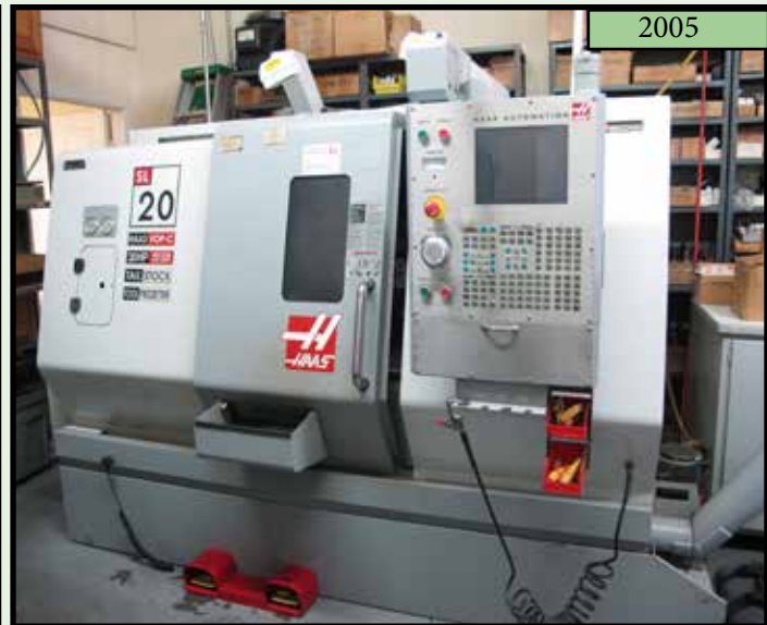
HAAS SL-20T CNC TURNING CENTER, TAIL STOCK, TOOL PRESETTER, 20HP VECTOR DRIVE, 8" CAPACITY CHUCK, CHICK AUGER, S/N 71179.
