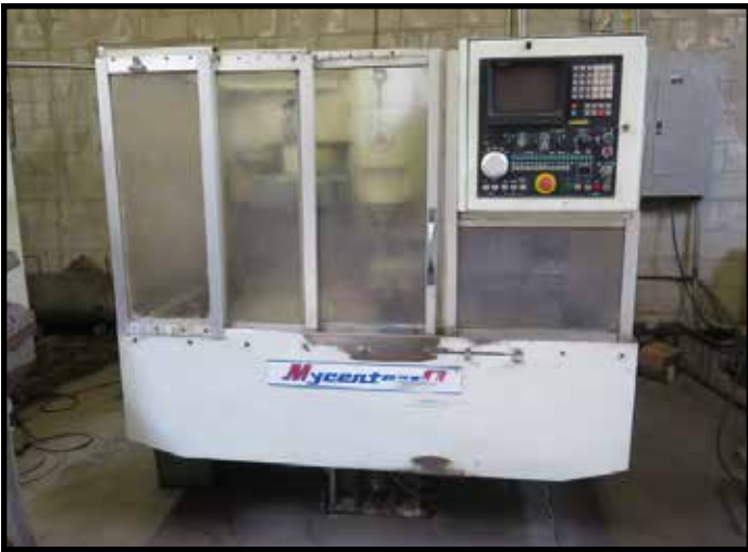
Kitamura MyCenter-0 CNC Vertical Machining Center w/ Fanuc 10M Controls
