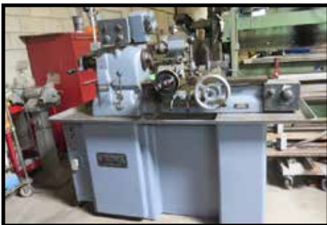
Hardinge Hand Chucker w/ Threading Attachment
