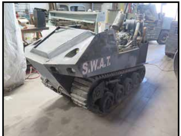
PAV Personal Assault Vehicle w/ 1/2" Armored Shell
