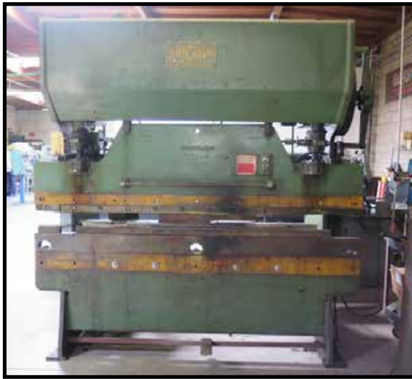
Chicago 68-B 36-55 Ton x 8' Press Brake w/ Controlled Back Gaging
