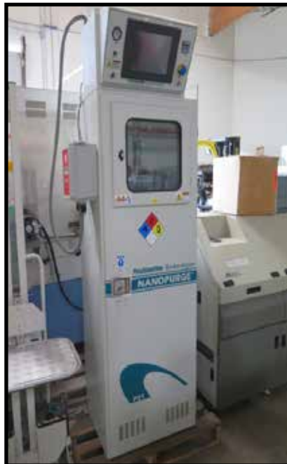
Precision Flow Technologies Gas Delivery System
