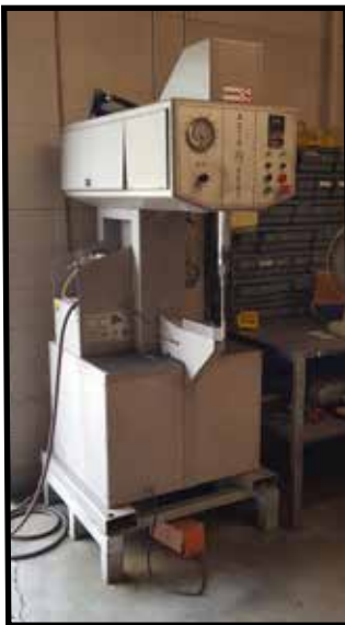
AUTO SERT AS-7.5 HYDRAULIC INSERTION PRESS WITH BOWL FEED, S/N 00337.
