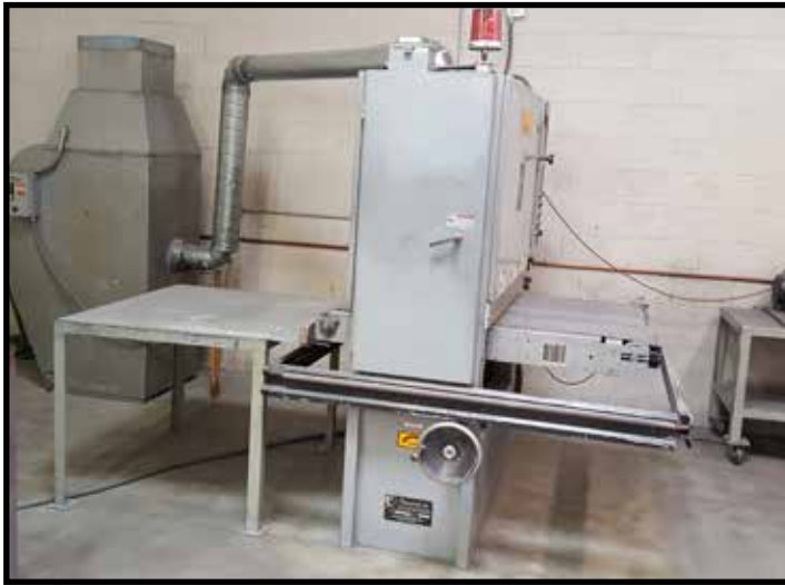
IMESAVER 137, 37" WIDE BELT GRAINDER WITH DUST COLLECTOR, S/N 23819M.
