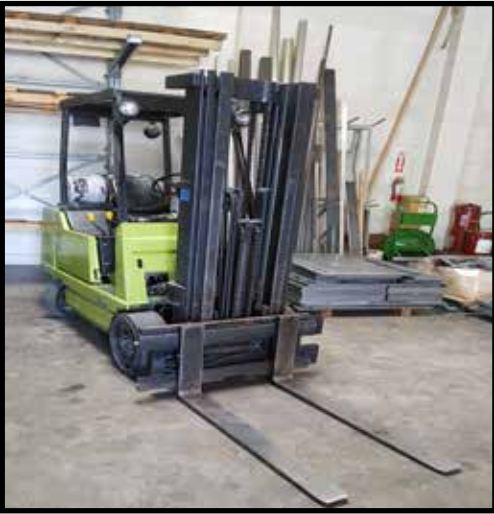
CLARK GC30MA, 6000 LB LPG FORKLIFT WITH SIDE SHIFT, 3 STAGE.
