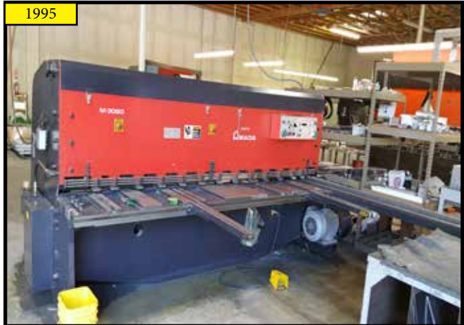
1995 AMADA M-3060, 10FT X .25" MECHANICAL POWER SHEAR WITH CNC BACK GAGE, S/N 30600919.
