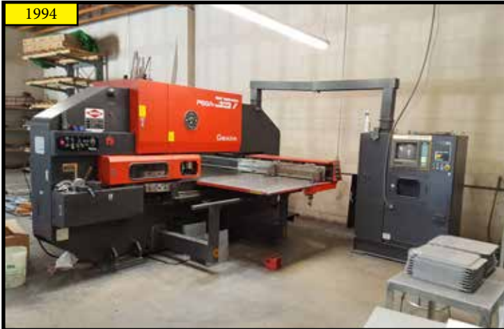
1995 AMADA PEGA 357 CNC TURRET PUNCH, 33 TON CAP, FANUC O4PC CONTROL, THICK TURRET, AUTO INDEX, 58 STATION TURRET, S/N AA570565.
