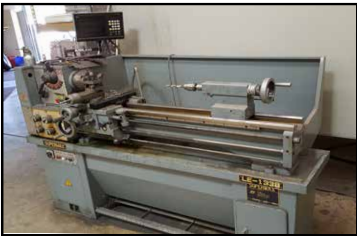
SUPERMAX LE-1338, 13" X 38" ENGINE LATHE WITH DRO.
