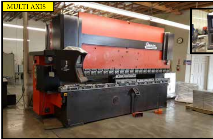
1993 AMADA HFBO-170- 40, 10FT X 187 TON CNC MULTI AXIS PRESS BRAKE, WITH OPERATEUR AMADA CONTROL, S/N A170-40- H31004.
