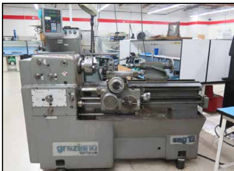
Graziano Tortona SAG12 12" x 32" Geared Head Lathe w/ Newall C80 DRO
