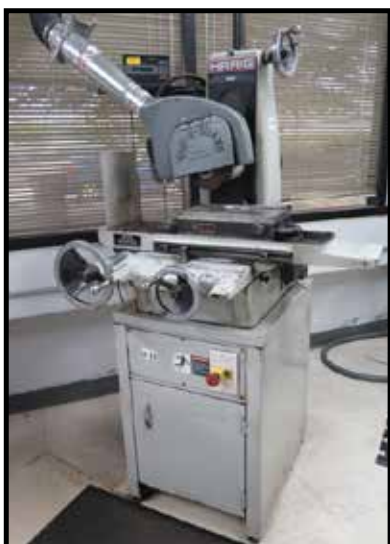
Harig mdl. 612 6" x 12" Surface Grinder w/ Acu-Rite DRO
