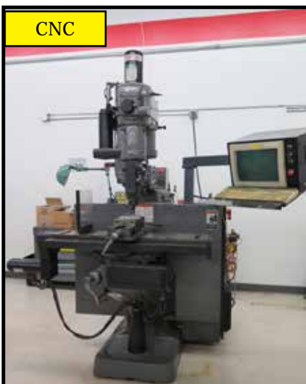
Bridgeport 3-Axis CNC Vertical Mill w/ BOSS PC Based CNC Controls
