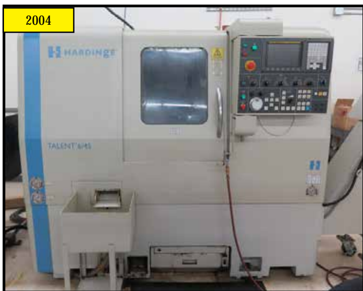
2004 Hardinge "Talent 6/45" Live Turret CNC Turning Center w/ Fanuc Oi-TB Controls
