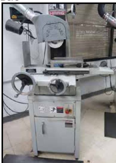
Harig mdl. 612 6" x 12" Surface Grinder w/ Acu-Rite Qwikcount DRO
