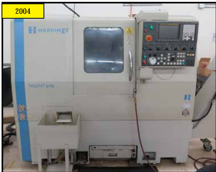
2004 Hardinge "Talent 6/45" Live Turret CNC Turning Center w/ Fanuc 0i-TB Controls
