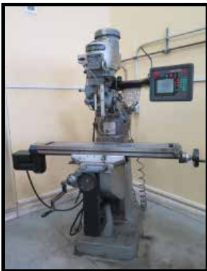
2000 Bridgeport / Proto Trak 2-Axis CNC Vertical Mill w/ Proto Trak EDGE Controls
