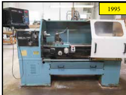
1996 TRAK TRL1745S 17" x 45" CNC Lathe w/ 2016 Upgraded Proto Trak SL Controls
