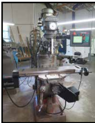
Alliant / Proto Trak 2-Axis CNC Vertical Mill w/ 2016 Upgraded Proto Trak EDGE Controls
