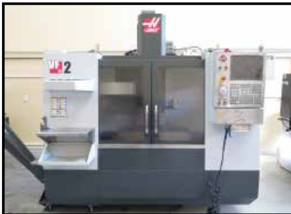
2012 Haas VF-2 CNC Vertical Machining Center w/ Haas Controls, 20 ATC, CAT-40 Spindle, 8100 RPM “AUCTION #2”
