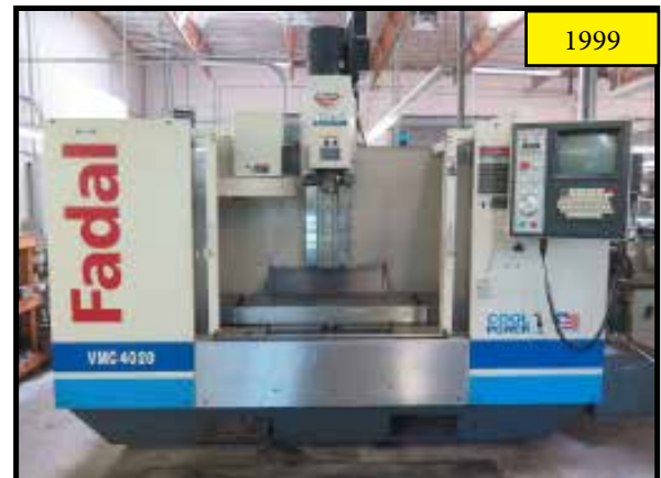
1999 Fadal VMC4020HT CNC Vertical Machining Center w/ Fadal Controls, 30-ATC, CAT-40 Spindle, 10,000 RPM, 28” Extended “Z” Axis “AUCTION #1”
