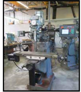
Alliant / Proto Trak 2-Axis CNC Vertical Mill w/ 2016 Upgraded Proto Trak EDGE Controls
