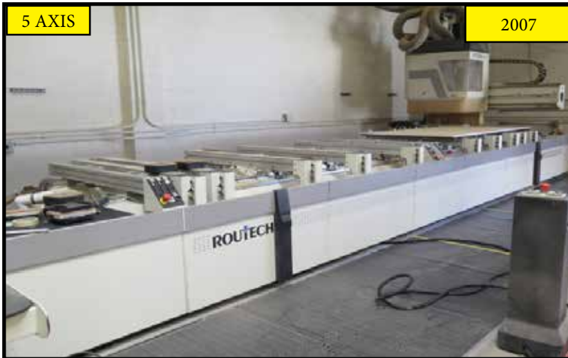
2007 Routech "Action Line" mdl. Record 110 AL PRISMA 5-Axis CNC Router s/n AA1-0162264 w/Routech Routolink PC Based Software and Control Package, 16-Station ATC, HSK-63 Taper Spindle, 49" x245" Work Area, (14) Adjustable Work Supports, Auto Clamping Devises, Vacuum Clamping Fixtures,Becker 7.5kW High Volume Vacuum Pump, Dust Conveyor.
