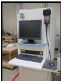
2007 Routech "Action Line" mdl. Record 110 AL PRISMA 5-Axis CNC Router s/n AA1-0162264 w/Routech Routolink PC Based Software and Control Package, 16-Station ATC, HSK-63 Taper Spindle, 49" x245" Work Area, (14) Adjustable Work Supports, Auto Clamping Devises, Vacuum Clamping Fixtures,Becker 7.5kW High Volume Vacuum Pump, Dust Conveyor.
