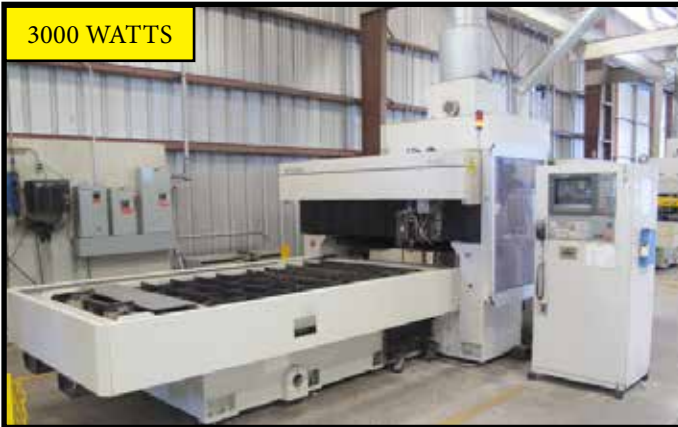
1996 Mitsubishi ML2512HD CNC Laser Processing Machine s/n 6625HD174 w/ Mitsubishi LC10BV Controls, Hand Wheel, 3000 Watt Laser, Mitsubishi ML4030D CO2 Laser Unit and Processing System
