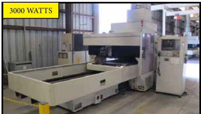
1998 Mitsubishi ML2512HD CNC Laser Processing Machine s/n ML1825HD224 w/ Mitsubishi Controls, Hand Wheel, 3000 Watt Laser, Mitsubishi mdl. 4030D CO2 Laser Unit and Processing System
