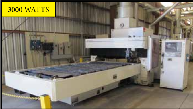
1996 Mitsubishi ML3015HD CNC Laser Processing Machine s/n 1630HD111 w/ Mitsubishi LC10BV Controls, Hand Wheel, 3000 Watt Laser, Mitsubishi ML4030D CO2 Laser Unit and Processing System
