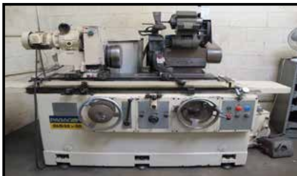
Paragon GUS32X50 Universal Grinder w/ Motorized Work Head with 9" Magnetic Chuck, OD and ID Grinding Heads, Hydraulic Feeds, Tailstock, Steady Rest
