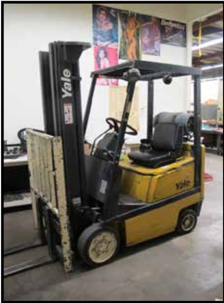
Yale 3000 Lb Cap LPG Forklift w/ 3-Stage Mast, 190" Lift Height, Side-Shift
