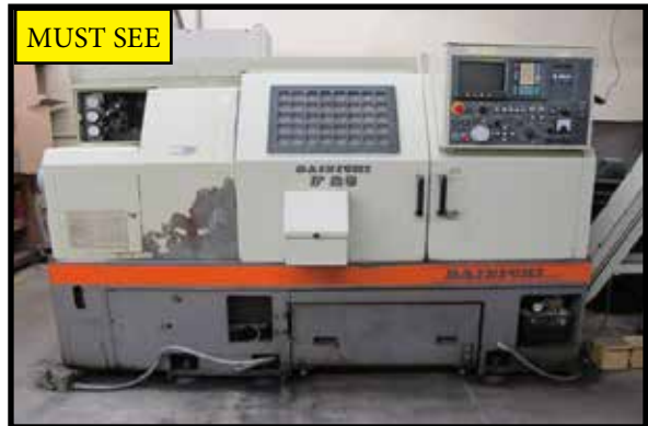
Dianichi F25 CNC Turning Center 25 X 600 w/ Fanuc Series 0-T Controls, 10-Station Turret, Tailstock, 10" 3-Jaw Chuck
