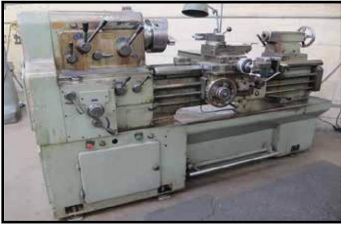
Cadillac mdl. 1733 17" x 33" Geared Head Gap Bed Lathe w/ 32-1800 RPM, Inch Threading, Tailstock, Steady Rest, Trava-Dial, 5C Collet
