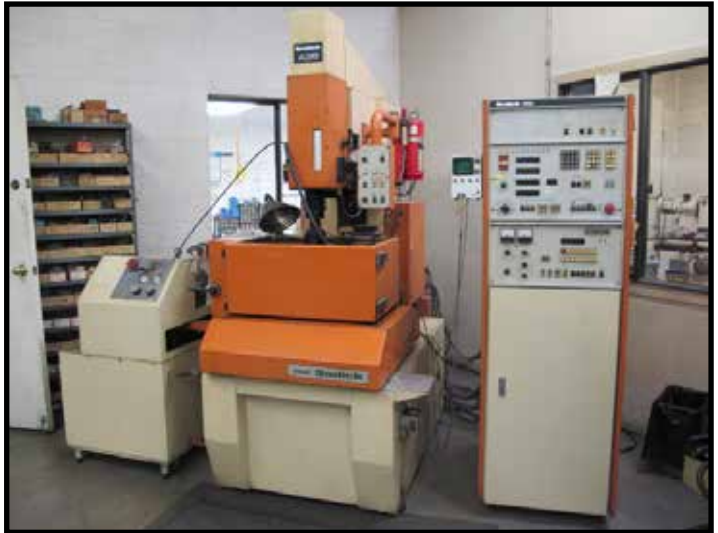
Sodick FS-A3B Die Sinker EDM Machine w/ Sodick 8100 Controls, System 3R Tooling System
