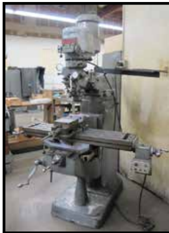
Bridgeport Series 1 - 2Hp Vertical Mill w/ 60-4200 Dial Change RPM, Power Feed
