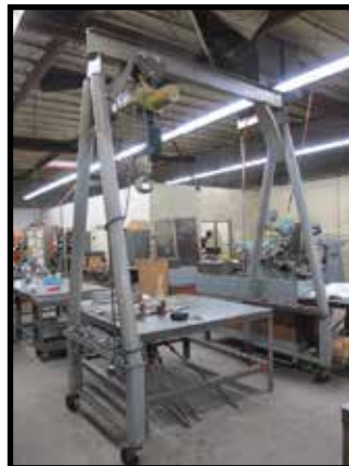
A-Frame Gantry w/ Yale 3-Ton Hoist
