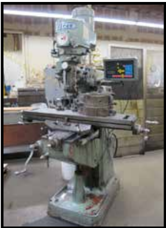
Sharp First mdl. LC-1 1/2 VH Vertical Mill w/ DRO II-2ML DRO, 3Hp Motor, 60-4500 Dial RPM, Chrome Ways
