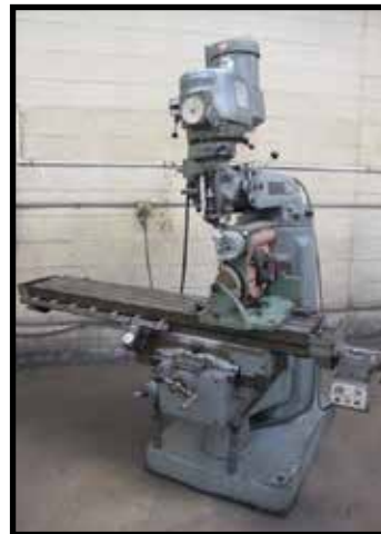
Bridgeport Series II Special Vertical Mill w/ 2Hp Motor, 60-4200 Dial Change RPM, Chrome Box Ways
