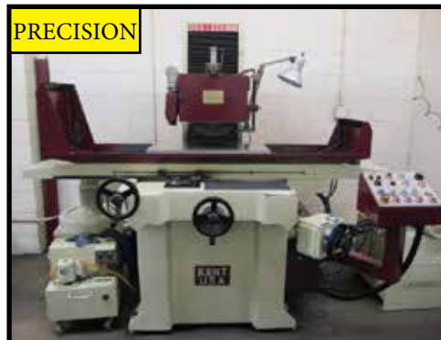
2009 Kent SGS-1230 AHD 12" x 30" Automatic Hydraulic Surface Grinder w/ Kent Controls, Automatic Cycles, Wheel Dresser
