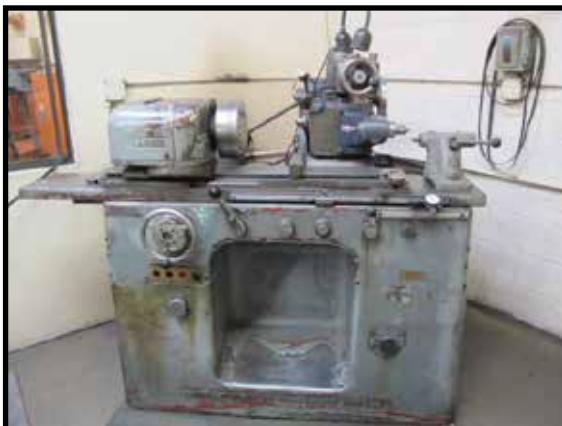
Landis 10" x 20" Universal Grinder w/ Motorized Work Head, OD and ID Grinding Heads
