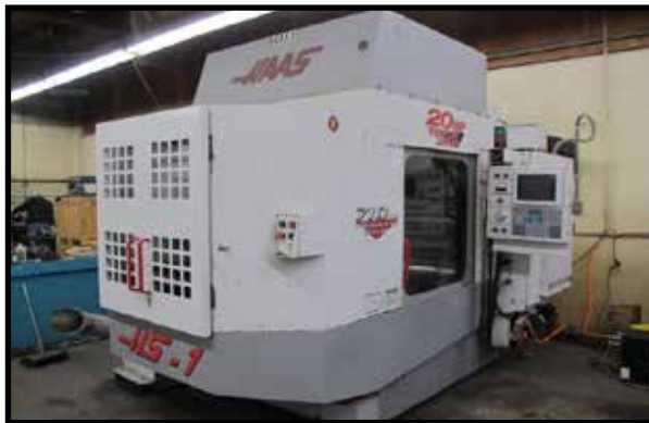
1998 Haas HS-1 4-Axis 2-Pallet CNC Horizontal Machining Center w/ Haas Controls, 24-Station ATC, CAT-40 Taper Spindle, 7500 RPM, 4 th Axis Thru Pallets, (2) 16" x 16" Pallets, 1mb Expanded Memory, Rigid Tapping, Coordinate Rotation and Scaling, Macros, Chip Auger, Haas Vector Spindle Drive
