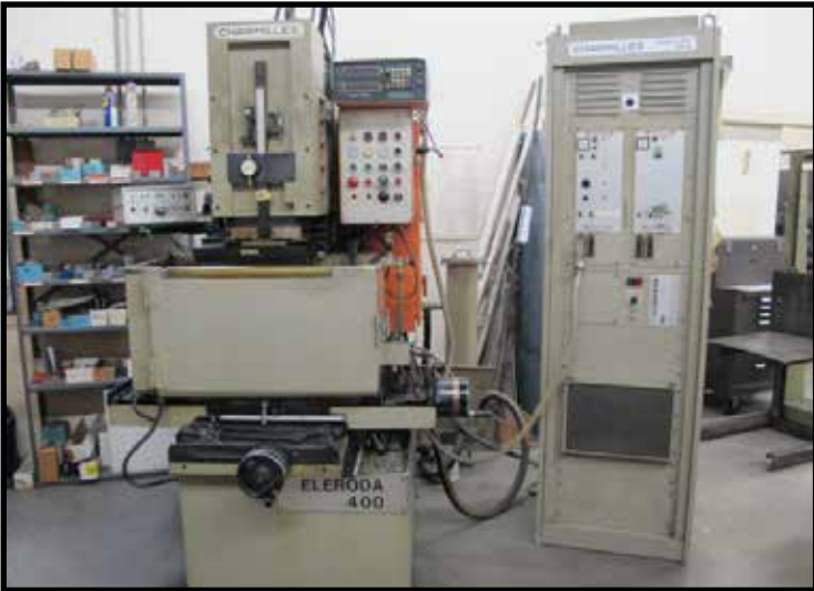
Charmilles Eleroda 400 Die Sinker EDM Machine w/ Charmilles Isopulse EP3 Controls, Acu-Rite II DRO
