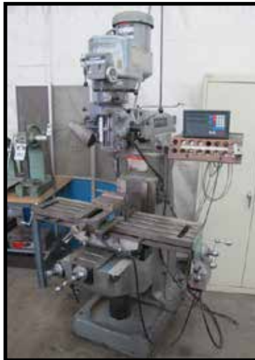
Bridgeport Vertical Mill w/ Newall DRO, 2Hp, 60-4200 Dial RPM, Chrome Ways, Power Feed
