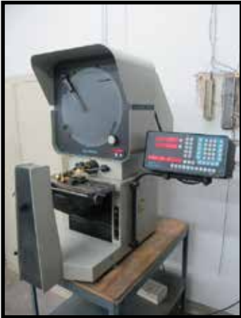
DELTRONIC DH214- MPC5E 14" OPTICAL COM- PARATOR W/ DELTRONIC MPC-5 PROGRAMMABLE DRO, DIGITAL ANGULAR READOUT,
