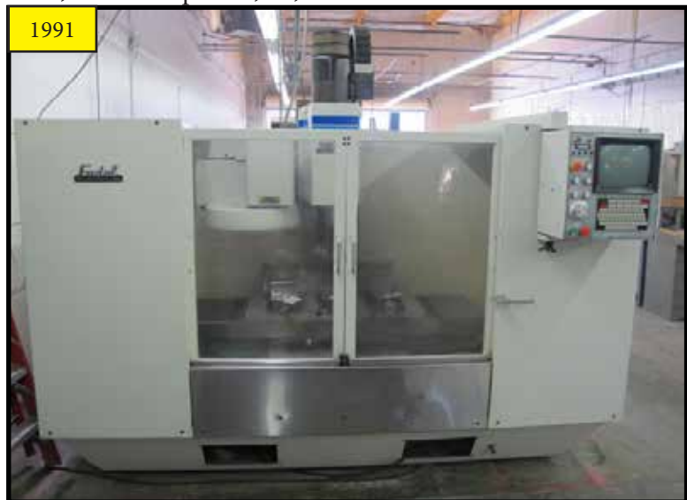
1991 Fadal VMC4020 mdl. 906-1 4-Axis CNC Vertical Machining Center w/ Fadal CNC88 Controls, 21-Station ATC, CAT-40 Spindle, 10,000 RPM
