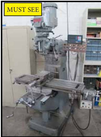
Bridgeport Series 1 2Hp Vertical Mill w/ Newall DRO, 60-4200 Dial RPM, Chrome Ways, Power Feed
