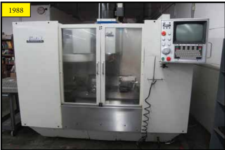
1988 Fadal VMC40 mdl. 904-1 4-Axis CNC Vertical Machining Center w/ Fadal CNC88 Controls, 21-Station ATC, CAT-40 Spindle, 10,000 RPM
