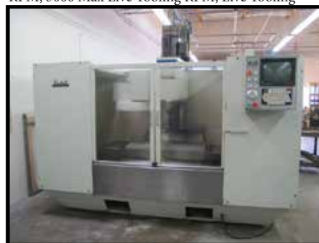
1987 Fadal VMC4020 mdl. 904-1 CNC Vertical Machining Center w/ Fadal CNC88 Controls, 21-Station ATC, CAT-40 Spindle
