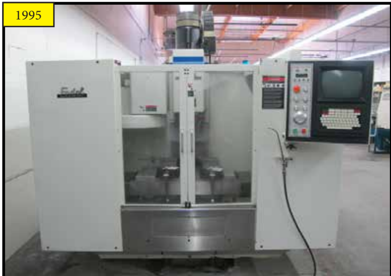
1995 Fadal VMC15RT mdl. 914-15 4-Axis CNC Vertical Machining Center w/ Fadal CNC88 Controls, 21-Station ATC, CAT-40 Spindle, Rigid Tapping
