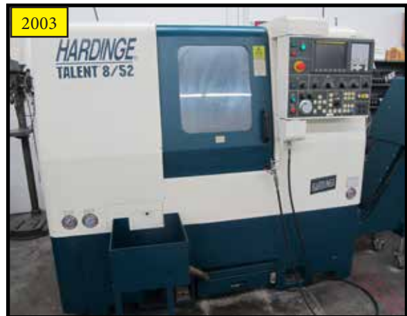
2003 Hardinge Talent 8/52 Live Turret CNC Turning Center w/ Fanuc Series 0i-TB Controls, Tool Presetter, 12-Station Live Turret, 5000 Max Spindle RPM, 5000 Max Live Tooling RPM, Live Tooling
